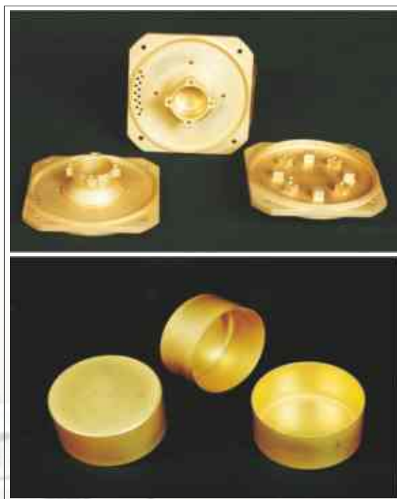
Microreaction wheel assembly parts of ISRO gold plated at CECRI
