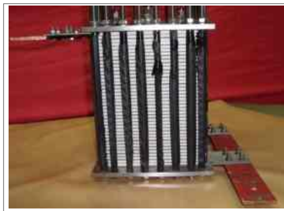
PEM Electrolyser of 3.0 Nm 3 /hr capacity
