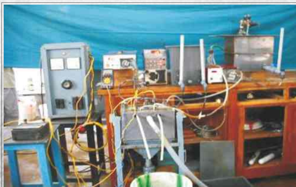
Electrolytic cell employed in the study
