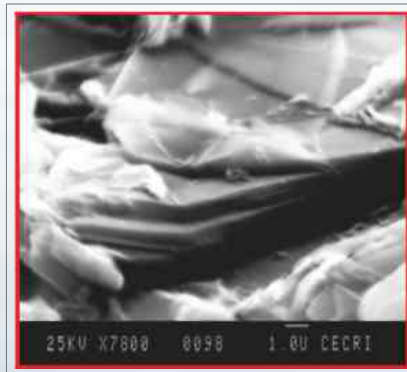
SEM image of kish graphite showing characteristic flaky morphology.
