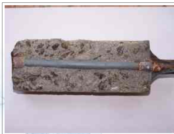
Broke-open concrete sample containing PMC coated reinforcement rod after 'time to cracking' study
