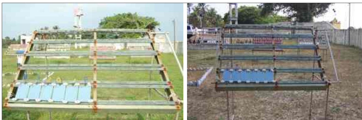
Painted panels at CECRI Atmospheric Corrosion Testing Centre, Mandapam. (a) Initial (b) After 2 months
