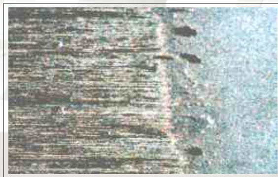
Optical micrographs of the worn surfaces of aluminum nitride coatings.
