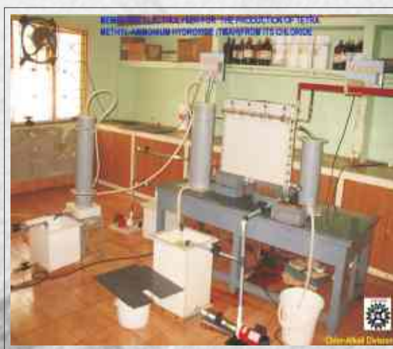
250A electrolyser for the production of TMAH
