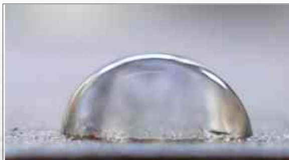
Contact angle of PTFE-silicone coating over steel.
