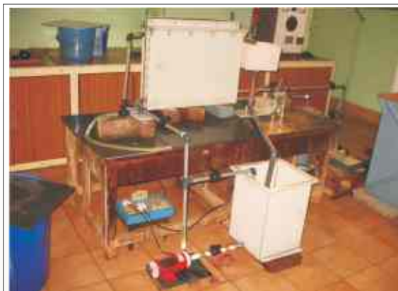
Membrane electrolyser of 250 A rating for the production of TBAH
