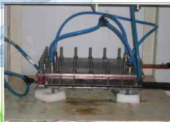
PEM Electrolyser of 2.0 Nm 3 /hr capacity
