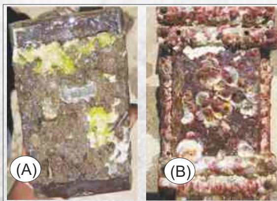
Surface of the SPGC-18 coating (A) exposed for 100 days in seawater; (B) exposed for 100 days in seawater & after seawater jetting for 3 minutes – only a portion of algae are removed
