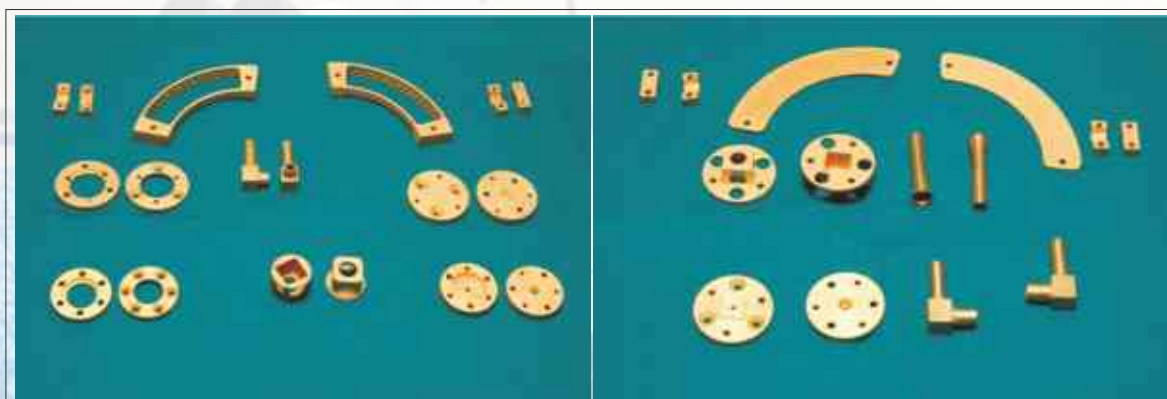
RWA and MWA minor parts of ISRO gold plated at CECRI
