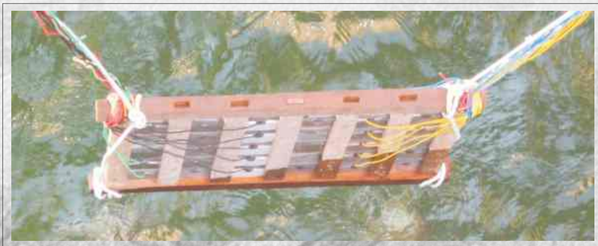
Specimens being immersed in sea for galvanic corrosion test
