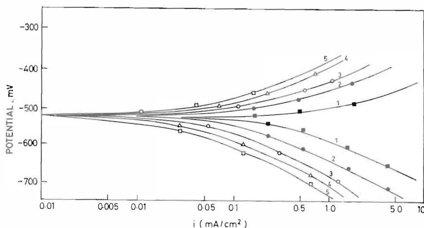
Fig. 2: Polarisation behaviour of iron in 1 N HCl with the addition of acid black II
