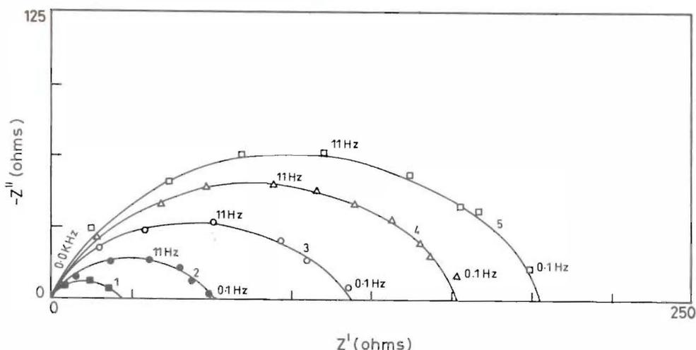
Fig. 3: Nyquist plots for iron in 1 N HCl with the addition of acid black II
