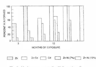
Fig. 1: Marine exposure studies W R on zinc alloys
