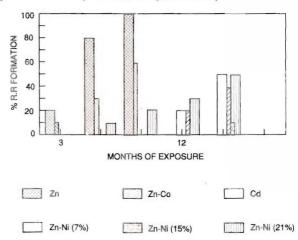
Fig. 3: Marine exposure studies R R formation of zinc alloys
