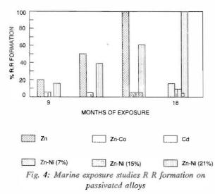
Cadmium and Zn-7% Ni behaved almost similarly upto 12 months and thereafter showed marked difference. Cadmium started rapid deterioration such that after 15 months its performance was equal to that of the 21% nickel alloy. Zn-15% alloy showed only 10% coverage by rust after 15 months of exposure.
