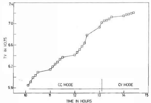
Fig. 2: Plot of battery voltage vs time
