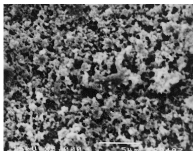
Fig. 3. SEM photograph of electrodeposited MoSe 2 thin film.
