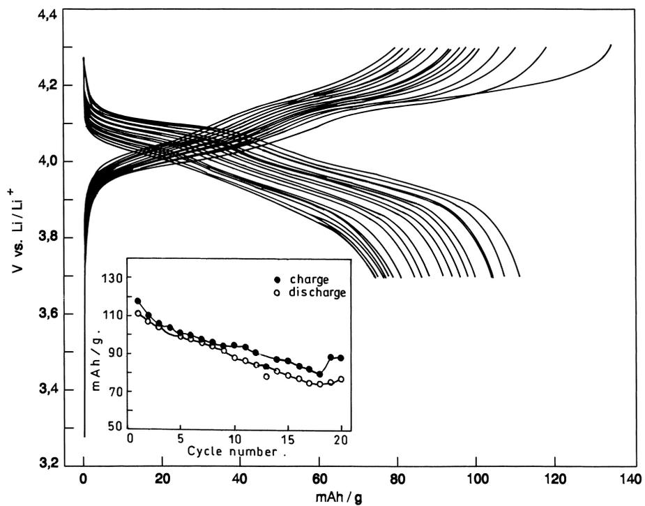
Fig. 4. Cycling behaviour of  $\text{LiTi}_{0.05}\text{Mn}_{1.95}\text{O}_4$ .
