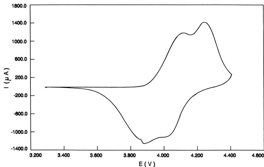
Fig. 3. Cyclic voltammogram of  $\text{LiTi}_{0.05}\text{Mn}_{1.95}\text{O}_4$ .
