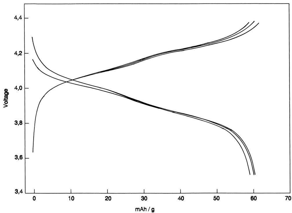
Fig. 6. Cycling behavior of LiMn<sub>2</sub>O<sub>4</sub> (synthesized at low temperature) coin cell.
