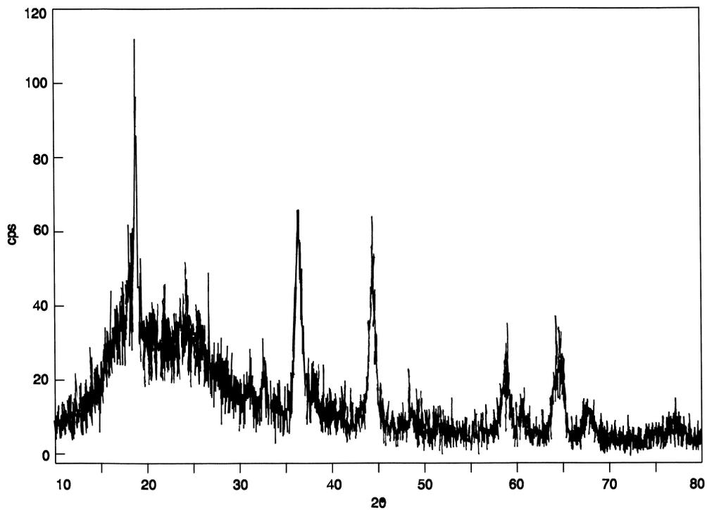
Fig. 5. X-ray diffraction of cycled  $\text{LiTi}_{0.05}\text{Mn}_{1.95}\text{O}_4$ .
