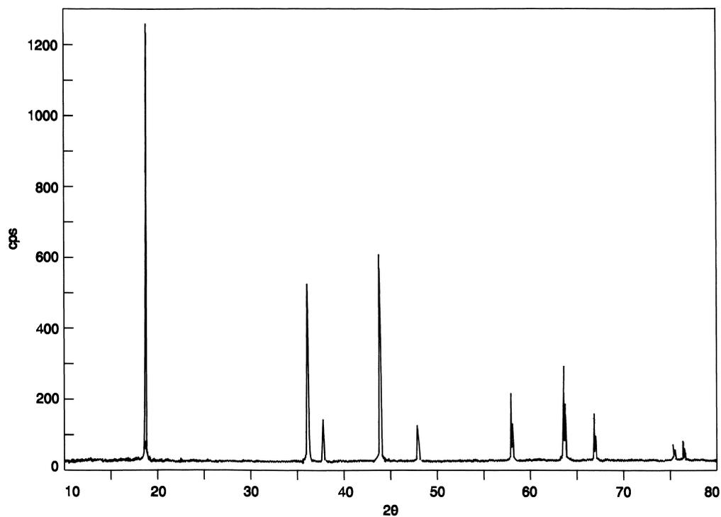
Fig. 1. X-ray diffraction of synthesized  $\text{LiTi}_{0.05}\text{Mn}_{1.95}\text{O}_4$ .
