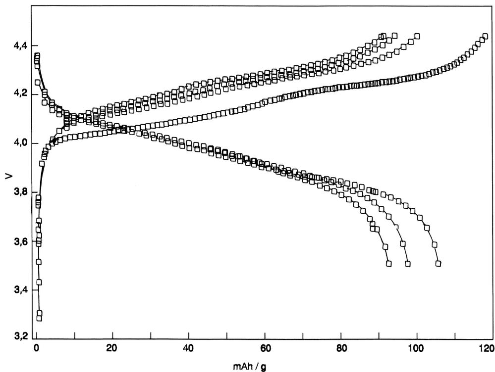
Fig. 7. Cycling behavior of LiTi<sub>0.05</sub>Mn<sub>1.95</sub>O<sub>4</sub>.
