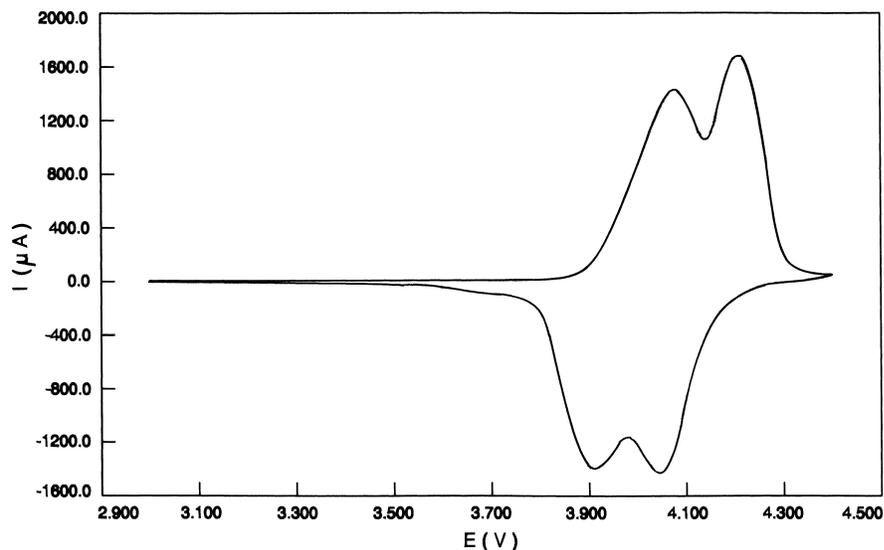
Fig. 2. Cyclic voltammogram of  $\text{LiMn}_2\text{O}_4$ .
