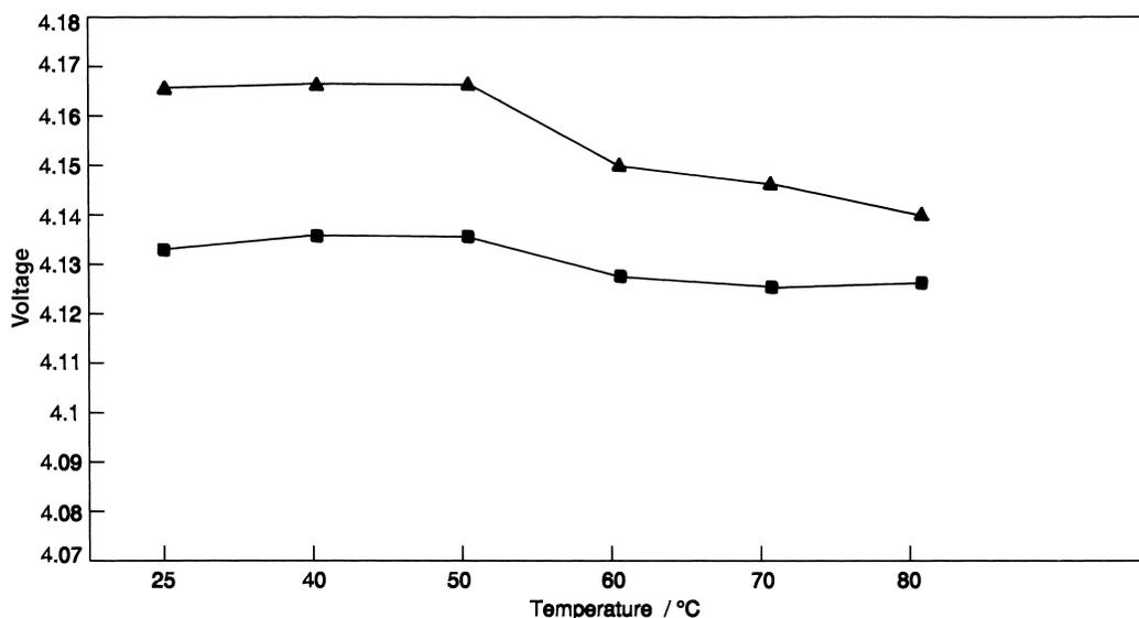
Fig. 8. Temperature dependence of open circuit voltage (OCV).
