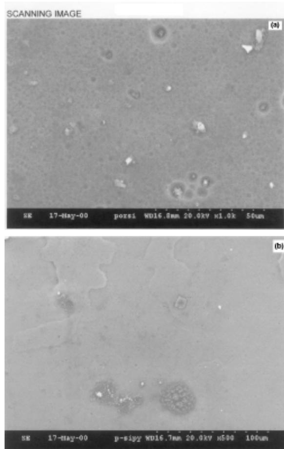
**Fig. 4.** SEM picture of (a) PSi and (b) PSi coated with polyaniline.
