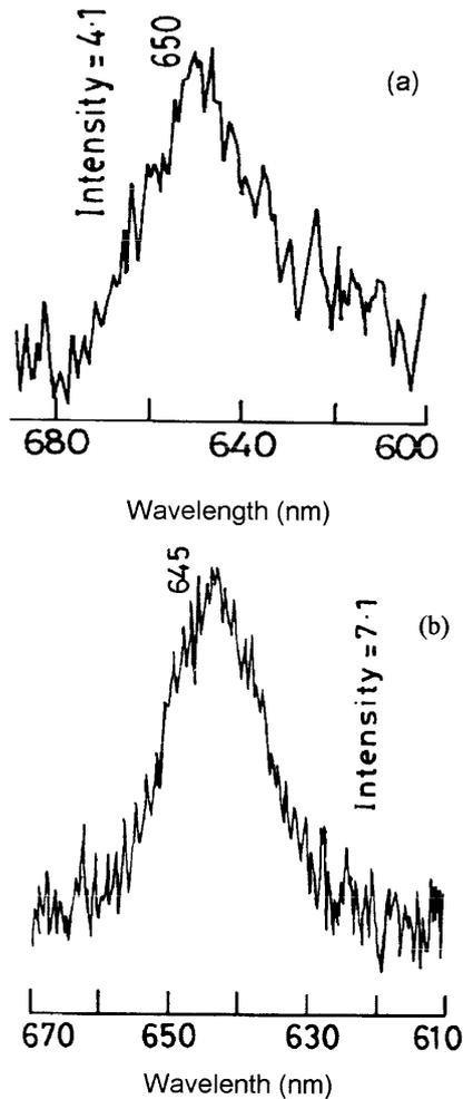
**Fig. 3.** Photoluminescence spectra of (a) polyaniline and (b) polyaniline filled PSi.
