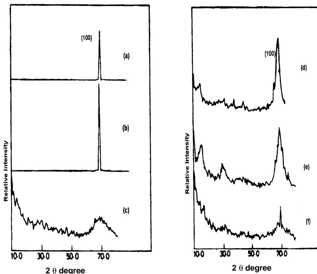
**Fig. 2.** XRD Spectra of (a) Crystalline silicon, anodized for 30 min at (b) 2 mA/cm<sup>2</sup>, (c) 10 mA/cm<sup>2</sup>, (d) 20 mA/cm<sup>2</sup>, (e) 45 mA/cm<sup>2</sup>, and (f) 60 mA/cm<sup>2</sup>.
