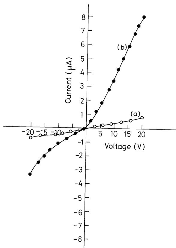
**Fig. 5.** Current-voltage characteristics of (a) Porous silicon surface and (b) Porous silicon surface coated with polyaniline.
