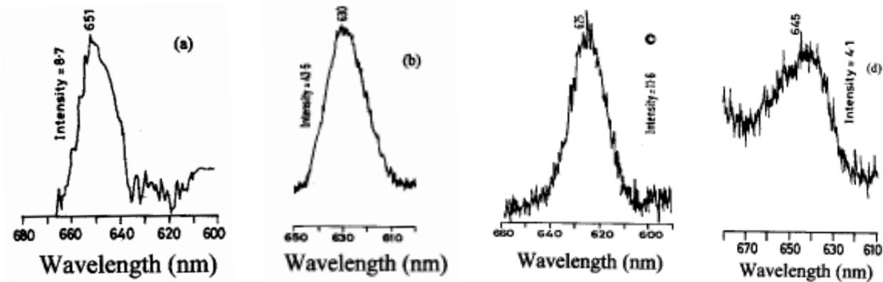
**Fig. 1.** Photoluminescence spectra of PSi formed at room temperature at 10 mA/cm<sup>2</sup>, (b) 20 mA/cm<sup>2</sup>, (c) 30 mA/cm<sup>2</sup>, and (d) 45 mA/cm<sup>2</sup>, for 30 minutes.
