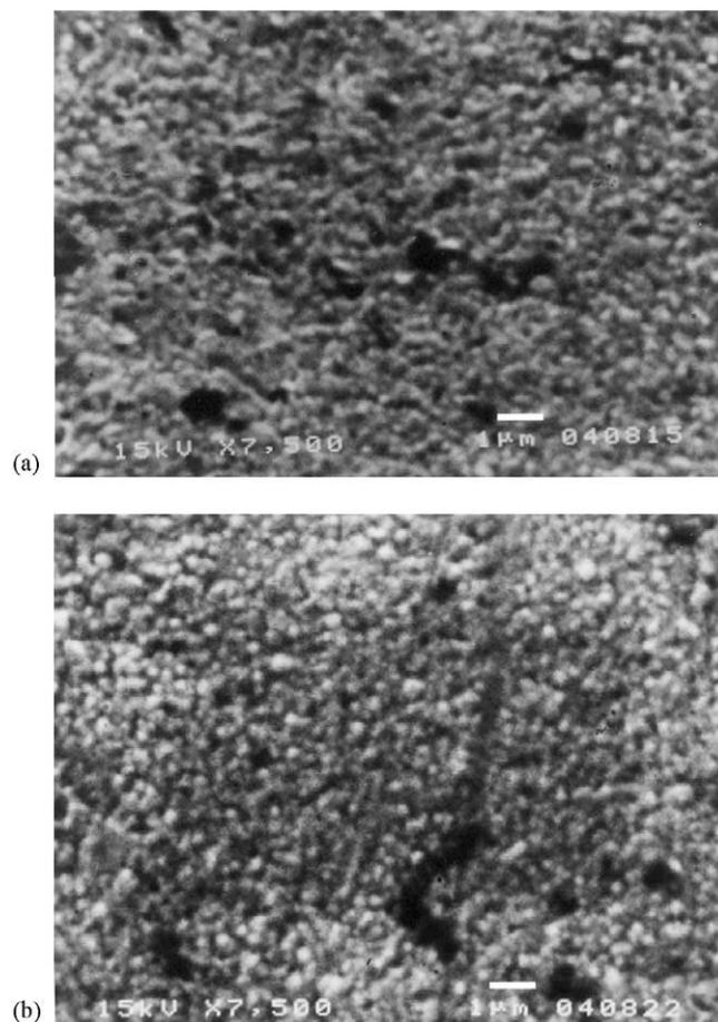
Fig. 7. Scanning electron micrographs of  $\text{WSe}_2$  thin films: (a) as prepared film; (b) film annealed at  $300^\circ\text{C}$  for 1 h.
