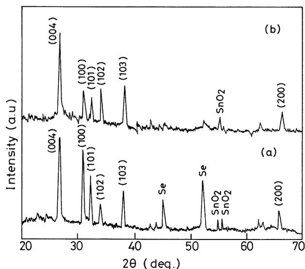
Fig. 3. XRD pattern of  $\text{WSe}_2$  thin films at optimised condition: (a) as-deposited; (b) annealed at  $300^\circ\text{C}$  for 1 h.
