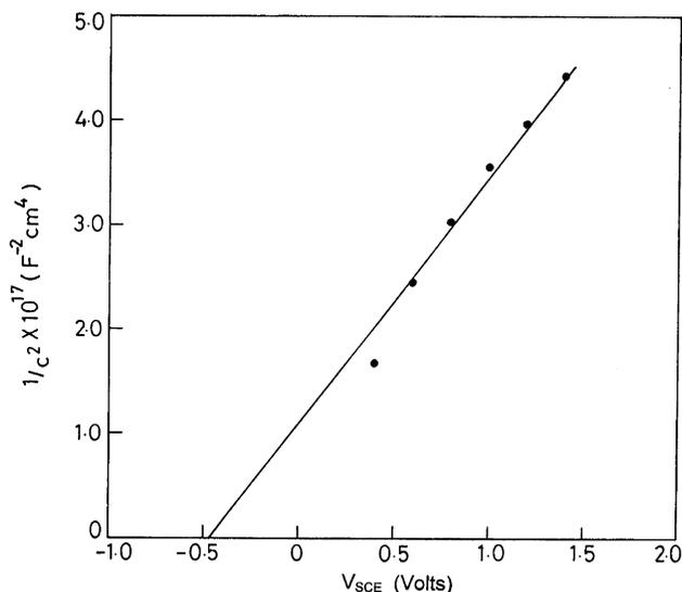
Fig. 6. Capacitance–voltage ( $V_{\text{SCE}}$ ) plot for  $\text{WSe}_2$  thin film in 0.2M,  $\text{Na}_2\text{SO}_4$  electrolyte.
