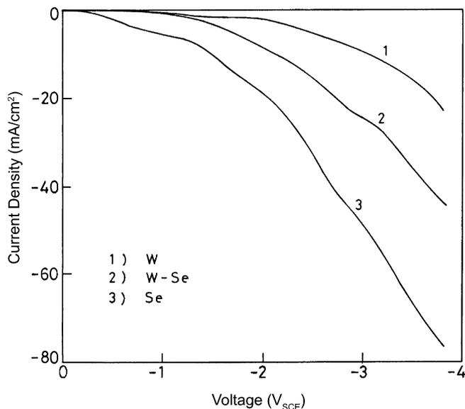
Fig. 1. Linear polarisation curves for W, Se, W–Se systems at 70 °C.
