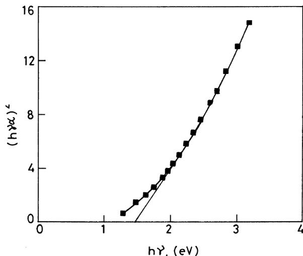
Fig. 5. Photon energy ( $h\nu$ ) vs.  $(\alpha h\nu)^2$  curve for  $\text{WSe}_2$  thin film.
