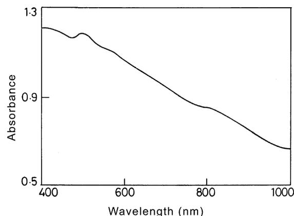
Fig. 4. Absorption spectrum of  $\text{WSe}_2$  thin film.
