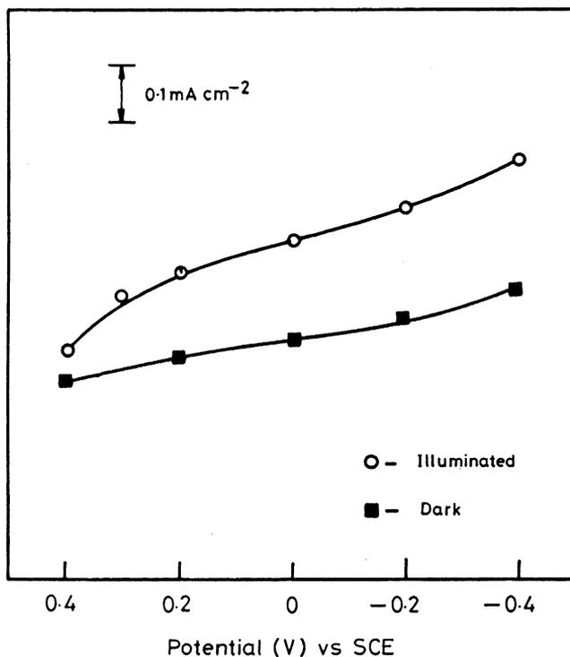
Fig. 3. Current–voltage ( $I$ - $V$ ) characteristics of the brush plated SnS film.
