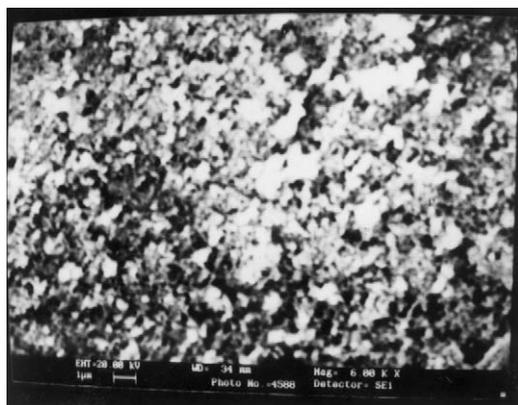
Fig. 2. Surface morphology of the brush plated SnS film.
