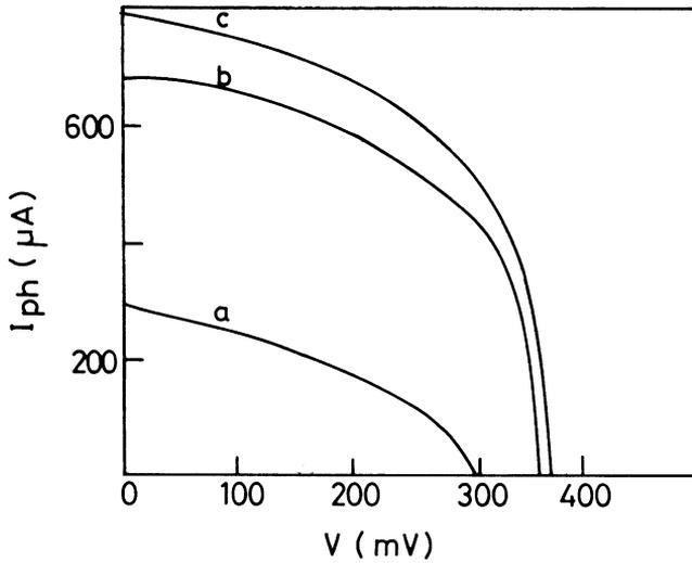
Fig. 6. Plot of power output characteristics for a typical p-SnS/Fe<sup>3+</sup>, Fe<sup>2+</sup>/Pt PEC solar cell.
