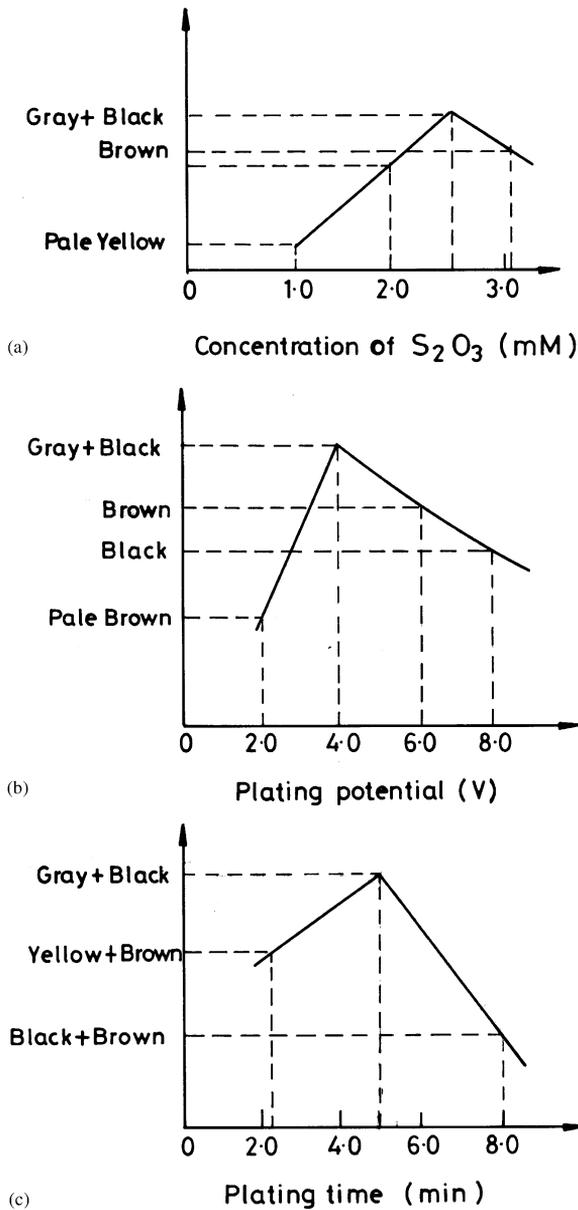
Fig. 1. Primary color observations for different plating parameters on brush plated SnS films (a) concentration of  $S_2O_3$ , (b) plating potential, (c) plating time
