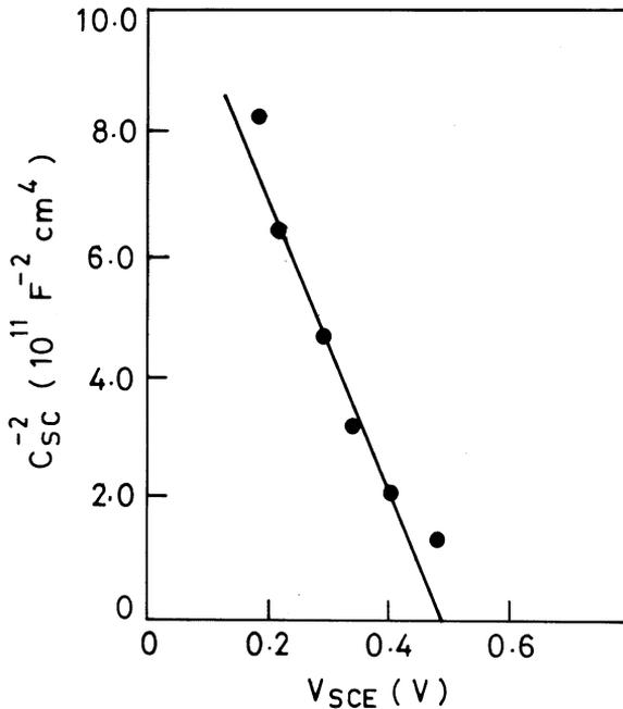
Fig. 4. Mott-Schottky plot for a brush plated SnS film.
