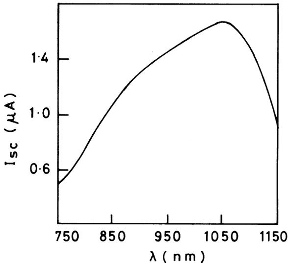
Fig. 5. Spectral response of SnS photoelectrode.
