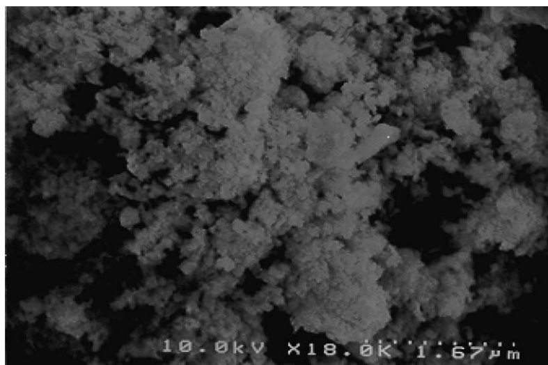
Fig. 3. SEM photograph of the \text{LiNi}_{0.5}\text{Mn}_{0.5}\text{O}_2 synthesized at 850°C.
