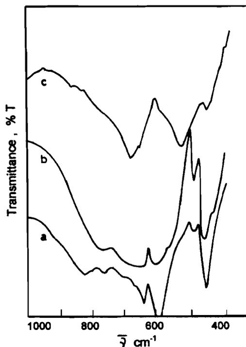
Fig. 4. FTIR for  $MgAl_2O_4$  sintered at (a) green, (b) 1000 °C (c) 1550 °C.
