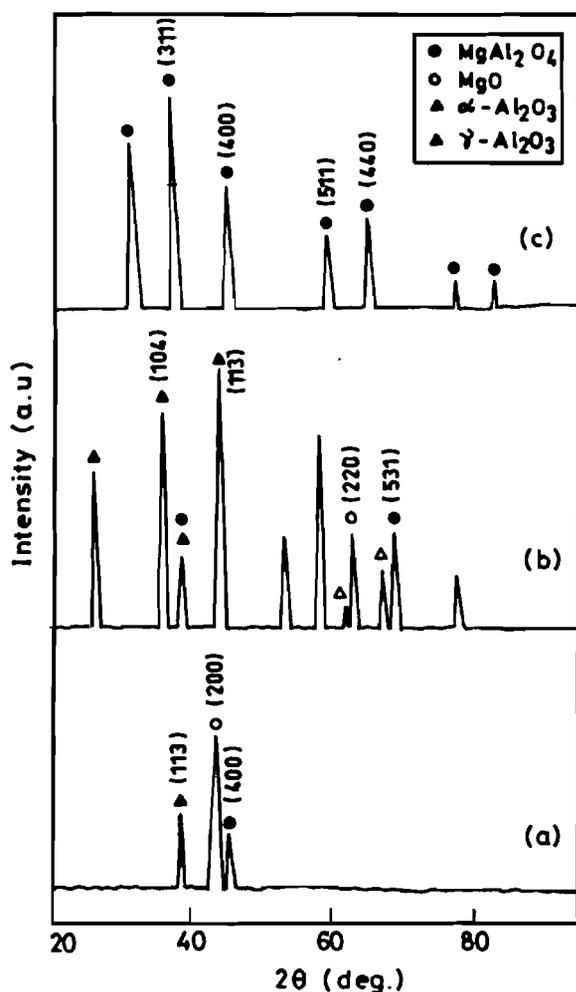
Fig. 3. XRD for  $MgAl_2O_4$  sintered at (a) green, (b) 1000 °C (c) 1550 °C.
