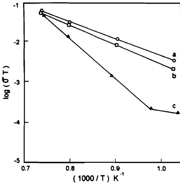
Fig. 1. Plot of  $\log(\sigma T)$  vs.  $10^3/T \text{ K}^{-1}$  for  $\text{MgAl}_2\text{O}_4$  sintered at (a) 973 K, (b) 1273 K, and (c) 1823 K.
