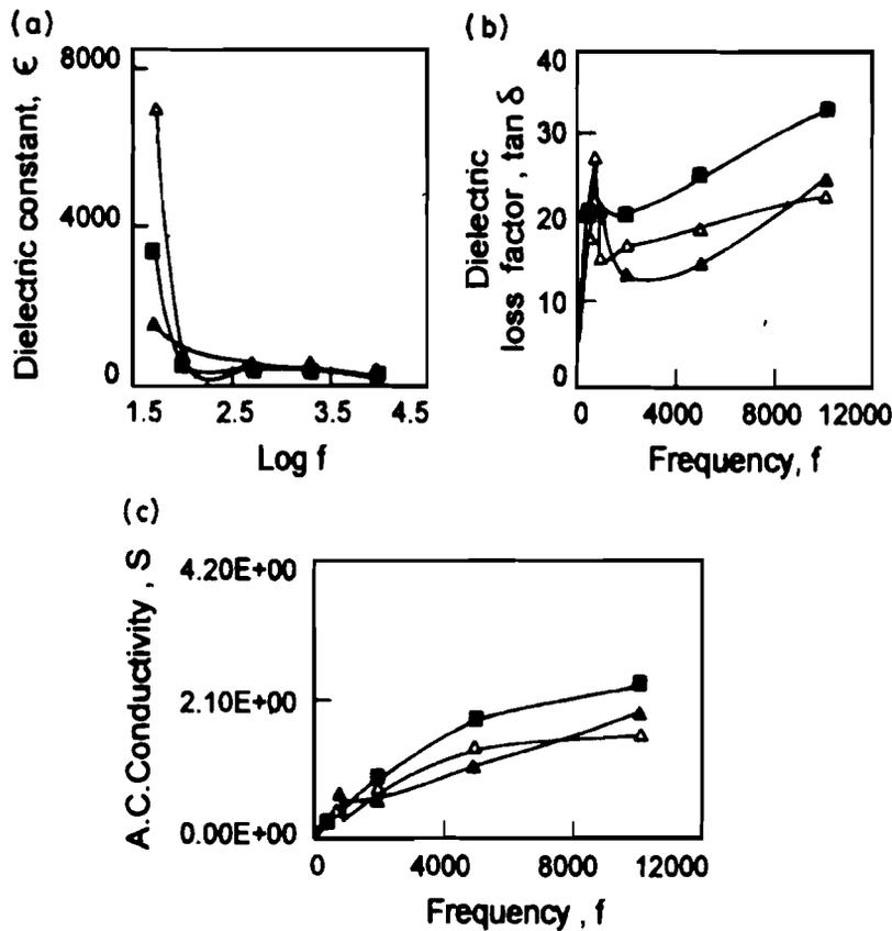
Fig. 2. Plot for (a) dielectric constant, (b) dielectric loss tangent and (c) AC conductivity of  $\text{MgAl}_2\text{O}_4$  sintered at  $\Delta$ - 30,  $\blacksquare$ - 700 and  $\blacktriangle$ - 1000 °C.
