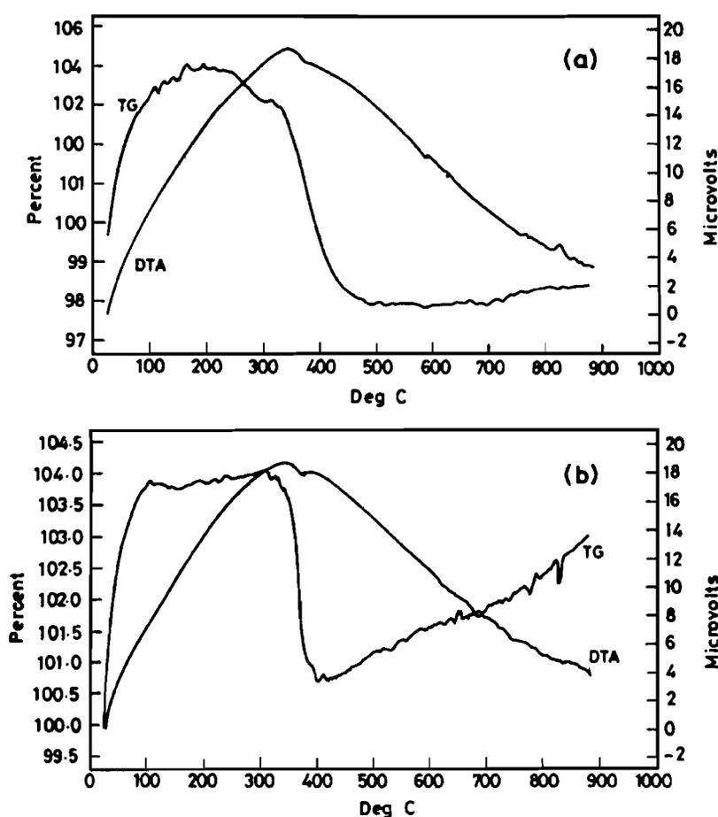
Fig. 5. TG/DTA curves for  $\text{MgAl}_2\text{O}_4$  sintered at (a) room temperature, (b)  $1550\text{ }^\circ\text{C}$ .
