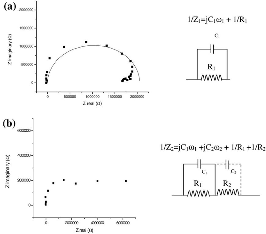
**Figure 6.** Nyquist impedance plot of LiNiVO<sub>4</sub> under (a) dark condition and (b) with UV (254 nm) exposure (· · · · ·: experimental; —: fitted).
