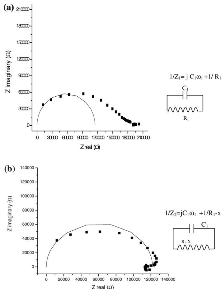
**Figure 5.** Nyquist impedance plot of  $\text{LiMn}_2\text{O}_4$  under (a) dark conditions and (b) with UV (254 nm) exposure (· · · · ·: experimental; —: fitted).
