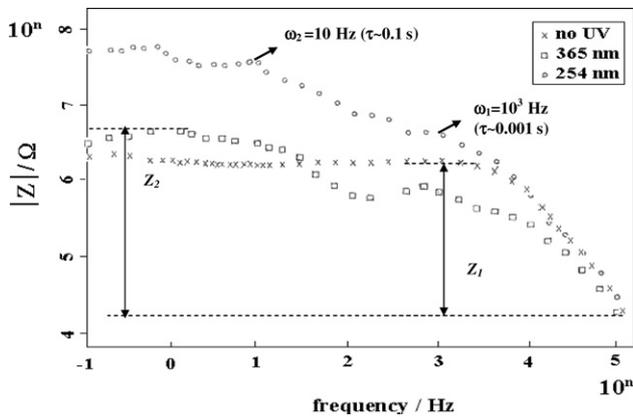
**Figure 4.** Bode impedance plots for the LiNiVO<sub>4</sub> pellet with and without UV irradiation. Total impedance  $Z_1$  (under no UV) and  $Z_2$  (under UV irradiation) and also time constants ( $\tau$ ) are indicated.
