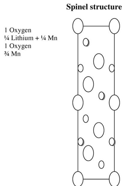
**Figure 2.** Normal spinel:  $\text{Li}[\text{Mn}_2]\text{O}_4$  (space-group:  $Fd\bar{3}m$ ): tetrahedral site:  $\text{Li}^+$ , octahedral site:  $\text{Mn}^{3+/4+}$ . Inverse spinel:  $\text{V}[\text{LiNi}]\text{O}_4$  (space-group:  $Fd\bar{3}m$ ): tetrahedral site:  $\text{V}^{5+}$ , octahedral site:  $\text{Li}^+$  and  $\text{Ni}^{2+}$ .
