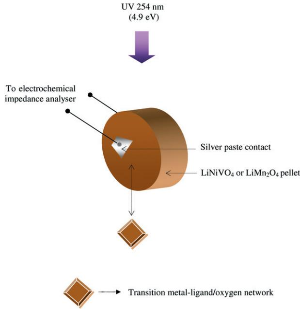
**Figure 1.** Schematic illustration of the photo-induced impedance measurement condition on the LiNiVO<sub>4</sub>/LiMn<sub>2</sub>O<sub>4</sub> pellet.
