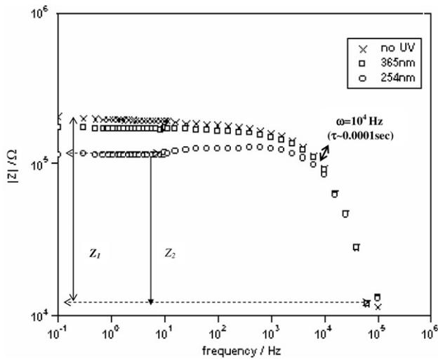
**Figure 3.** Bode impedance plots of LiMn<sub>2</sub>O<sub>4</sub> pellet with and without UV exposure. Total impedance  $Z_1$  (under no UV) and  $Z_2$  (with UV irradiation) are indicated.
