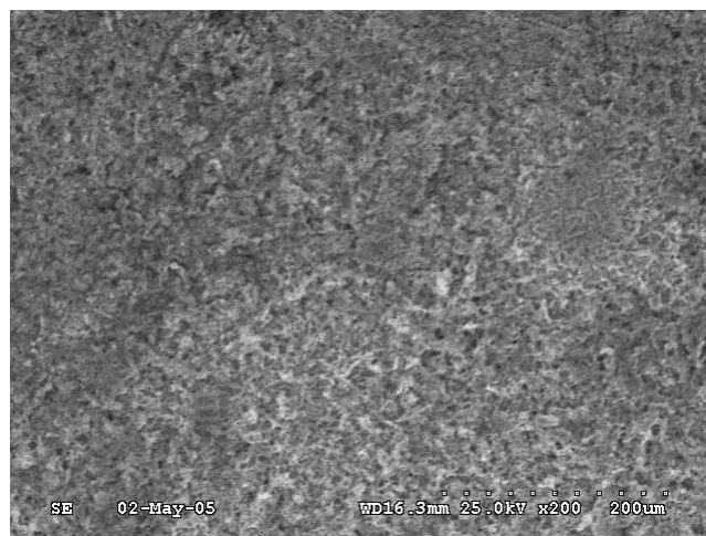
Fig. 9. SEM photograph for carbon steel dipped in 1 mol/L HCl with 200 mmol/L CTAB.
