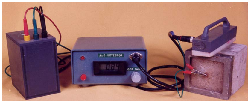
Fig. 4. Photograph of the galvanostatic pulse instrument with probe and concrete sample.
