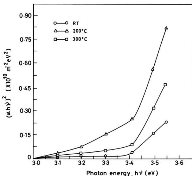
Fig. 5. The 'Tauc' plot of ZnO thin films deposited at RT, 200 °C and 300 °C.
