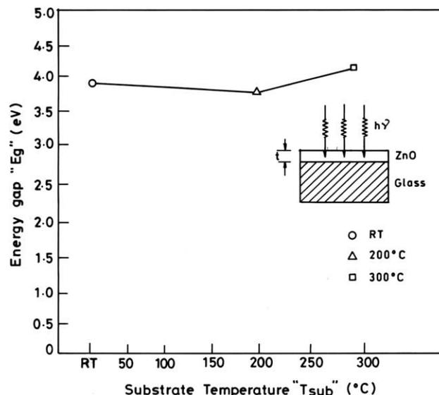
Fig. 6. The plot of energy gap ' $E_g$ ' of ZnO thin films versus substrate temperature  $T_{\text{sub}}$  (°C).
