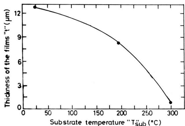
Fig. 4. The plot of thickness of ZnO thin films deposited at RT, 200 °C and 300 °C versus substrate temperature ' $T_{\text{sub}}$ ' (°C).
