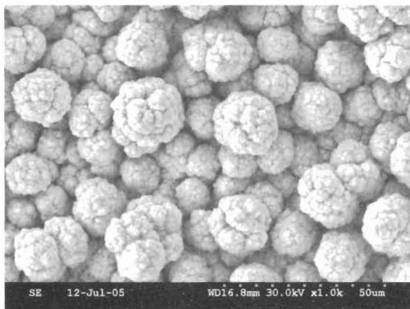
Fig. 4 : Effect of chloride addition on the Secondary electron image of Cr-Ni-Fe deposit at 1000 X, plated for 15 minutes duration at a CD of 60 mA/cm 2 , from solution containing Nickel acetate 10 g/l, Chromium acetate 24 g/l, Ferrus ammonium sulfate, 80 g/l, Boric acid 30 g/l, Ascorbic acid 60 g/l, Hydrochloric acid 4, 8 & 12 ml/l respectively, at 50°C
