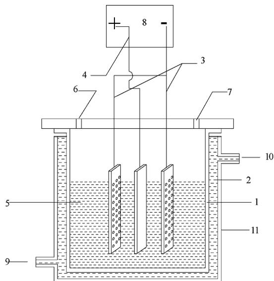
**Figure 1.** Schematic of the laboratory-scale cell assembly. Legend: 1, cell; 2, thermostatic water; 3, stainless steel cathode; 4, anode; 5, electrolyte; 6 & 7, holes to introduce pH sensor and thermometer; 8, dc source; 9, inlet; 10, outlet; and 11, thermostat.
