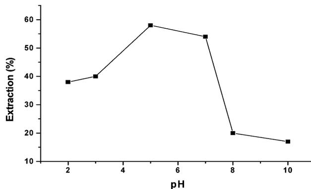
**Figure 2.** Effect of pH on the extraction efficiency of chromium. Conditions: electrolyte (NaCl) concentration, 30 g/L; volume, 400 mL; mass of sludge, 10 g; current density, 10 A/dm<sup>2</sup>; duration of electrolysis, 30 min.
