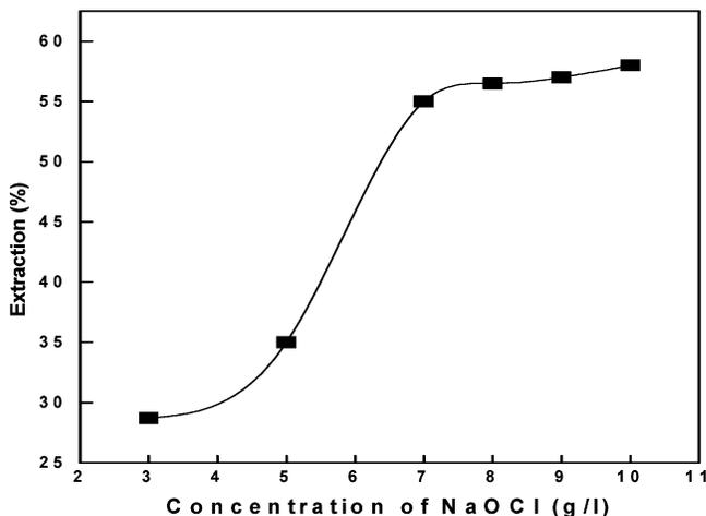
**Figure 3.** Effect of concentration of hypochlorite on extraction efficiency. Conditions: electrolyte (NaCl) concentration, 30 g/L; volume, 400 mL; pH, 5.0–5.5; mass of sample, 10 g; current density, 10 A/dm<sup>2</sup>; duration of electrolysis, 30 min.
