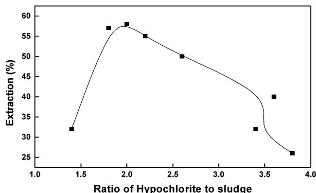
**Figure 4.** Effect of the ratio of hypochlorite to sludge on the extraction. Conditions: electrolyte (NaCl) concentration, 30 g/L; pH, 5.0–5.5; mass of sample, 10 g; current density, 10 A/dm<sup>2</sup>.
