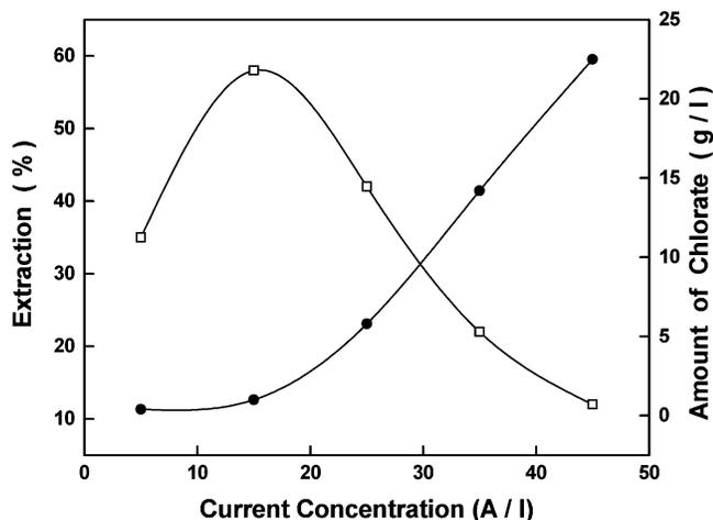
**Figure 5.** Effect of current concentration on extraction efficiency. Conditions: electrolyte (NaCl) concentration, 30 g/L; pH, 5.0–5.5; mass of sample, 10 g; current density, 10 A/dm<sup>2</sup>.
