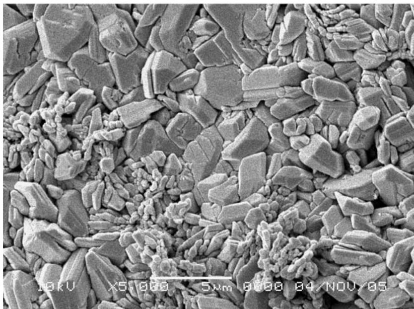
Fig. 19. Electrode surface morphologies of the cured conventional negative plate after treatment with PANI dissolved in oxalic acid solution.
