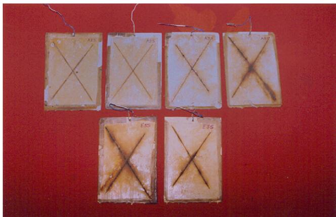
Fig. 5. Panels after immersion in NaCl solution (A2S, A3S and E3S).
