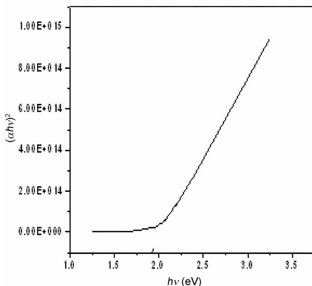
Figure 7. Band gap of CdSe at RT.
