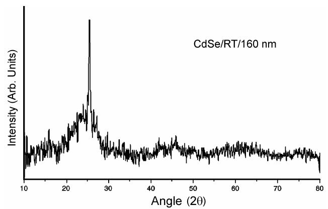
**Figure 4.** X-ray diffractogram of CdSe film of thickness, 160 nm.
