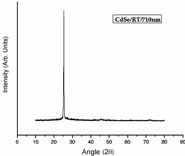
**Figure 2.** X-ray diffractogram of CdSe film of thickness, 710 nm.
