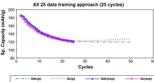
Fig. 6. Prediction (extrapolation) of extended cycle charge–discharge behavior—all 25 data (up to 25 cycles) training approach.
