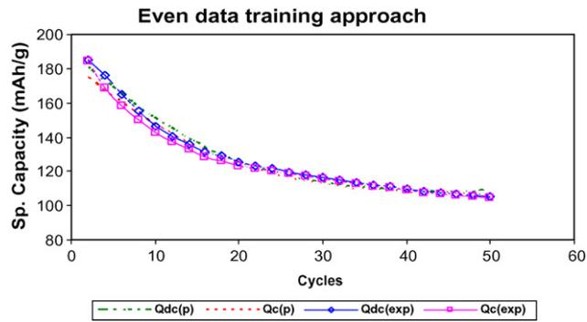
Fig. 3. Estimation (interpolation) of odd cycle charge–discharge behavior— even cycle data training approach.
