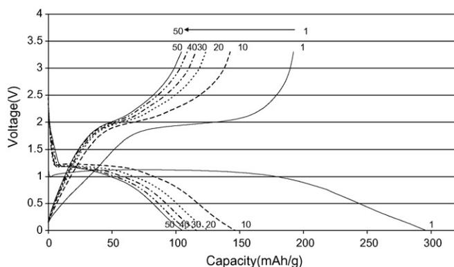
Fig. 1. Charge–discharge behavior of CoO.
