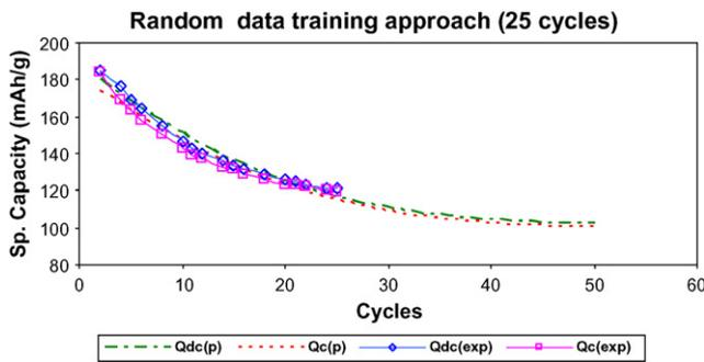
Fig. 5. Prediction (extrapolation) of extended cycle charge–discharge behavior—random data (up to 25 cycles) training approach.
