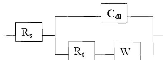
Fig. 6 — Equivalent circuit for AC impedance spectra
