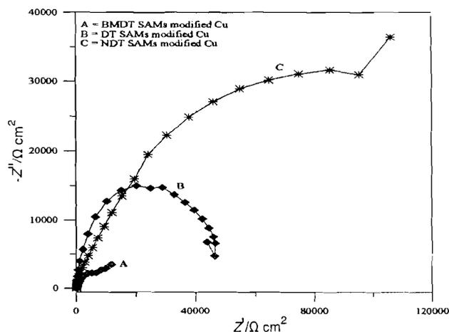
Fig. 5 — Nyquist impedance spectrum of DT, NDT and BDMT SAM modified Cu electrode in 0.5 M NaCl solution at open circuit potential. 10 mM solution of thiols in toluene was taken for SAM formation with a self-assembly period of 2 h
