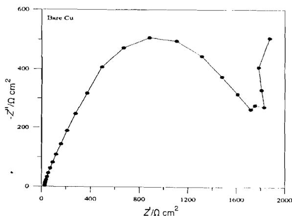
Fig. 4 — Nyquist impedance spectrum for the bare Cu electrode in 0.5 M NaCl solution at open circuit potential
