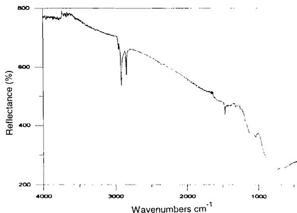
Fig. 7 — FT-IR reflection spectrum for DT/SAM on copper surface
