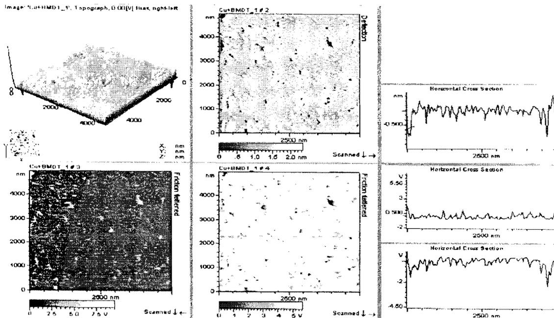
Fig. 14 — Typical topography (3-dimensional), deflection and friction images obtained for BMDT/SAM modified copper surface and their cross section analysis
