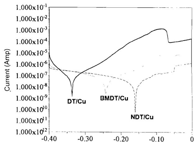
Fig. 3 — Potentiodynamic polarization of SAM modified copper with self-assembly period of two hours in 0.5 M NaCl solution at 0.01 Vs<sup>-1</sup>
