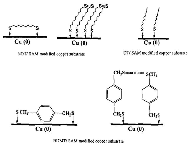
Fig. 10 — Self assembled monolayer of NDT, NDT and BDMT on oxide free copper substrate
