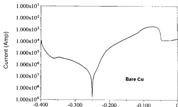
Fig. 2 — Potentiodynamic polarization of bare copper in 0.5 M NaCl solution at 0.01 Vs<sup>-1</sup>
