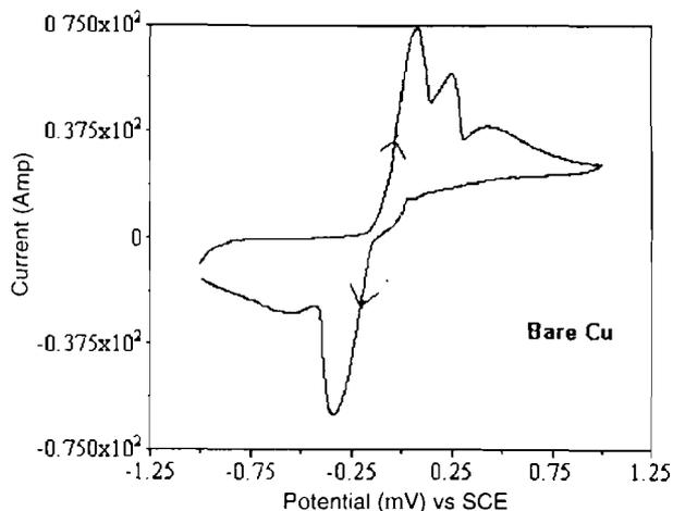
Fig.15 — Cyclic voltammogram of bare copper electrode in 0.5 M NaCl solution at a scan rate of  $20 \text{ mVs}^{-1}$
