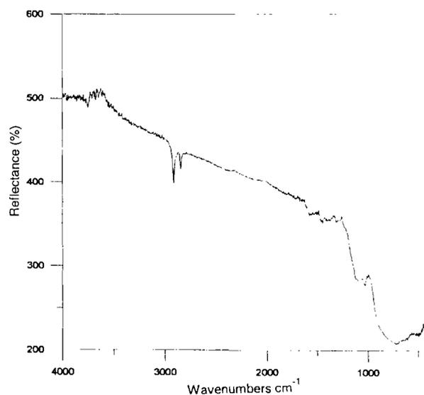
Fig. 8 — FT-IR reflection spectrum for NDT/SAM on copper surface
