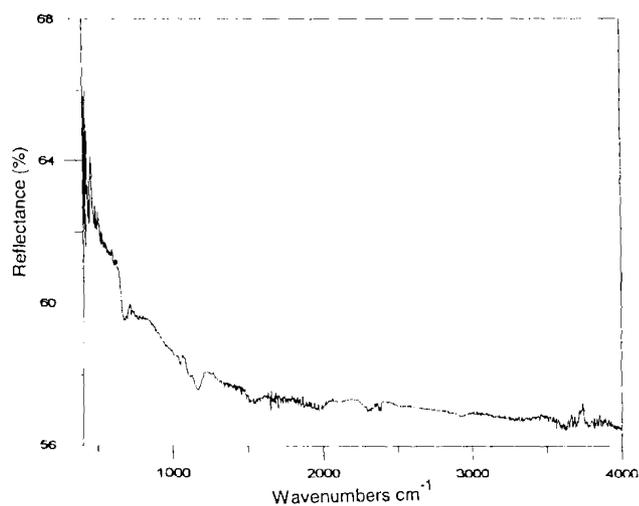
Fig. 9 — FT-IR reflection spectrum for BDMT/SAM on copper surface
