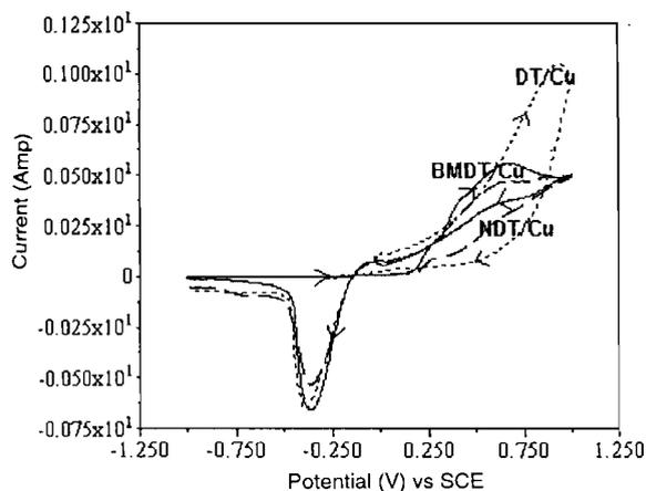
Fig. 16 — Cyclic voltammogram of BMDT, DT and NDT SAM modified copper electrode in 0.5 M NaCl solution at 20  $\text{mV}\cdot\text{s}^{-1}$  scan rate
