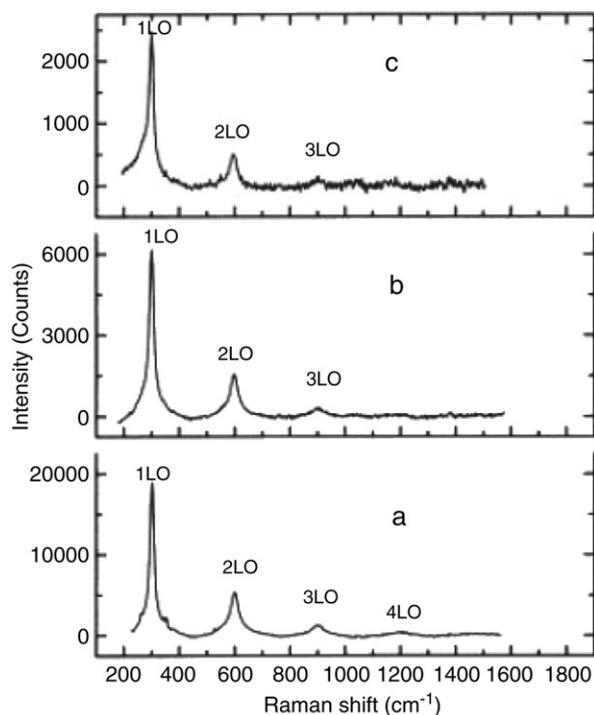
Fig. 5. Raman spectra of CdS films deposited on different substrate temperatures: (a) 5 °C, (b) 15 °C and (c) 30 °C.
