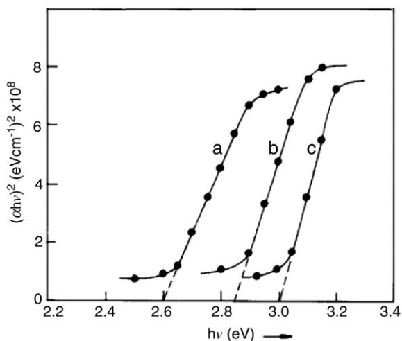
Fig. 3.  $(\alpha h\nu)^2$  vs.  $h\nu$  plot of CdS films deposited at different temperatures: (a) 30 °C, (b) 15 °C and (c) 5 °C.
