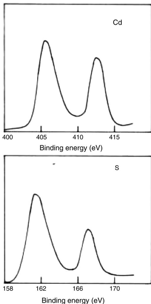
Fig. 2. XPS of CdS films deposited at 5 °C.
