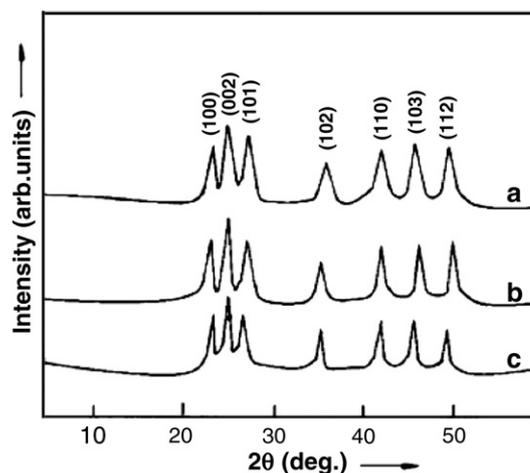
Fig. 1. XRD pattern of CdS films deposited at different temperatures: (a) 5 °C, (b) 15 °C and (c) 30 °C.
