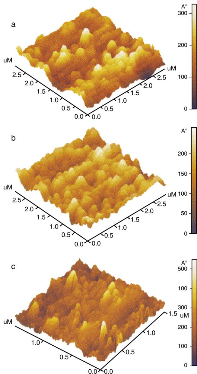
Fig. 4. Atomic force micrograph of CdS films deposited at different temperatures: (a) 30 °C, (b) 15 °C and (c) 5 °C.
