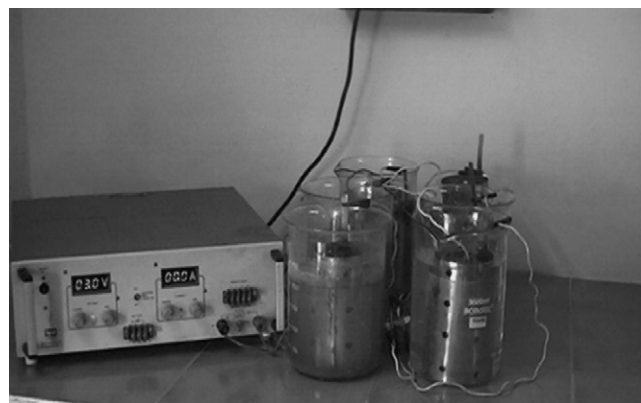
Fig. 2. Experimental setup for time to cracking study.
