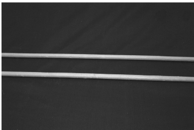
Fig. 10. Surface condition of rebar after cathodic disbondment test.
