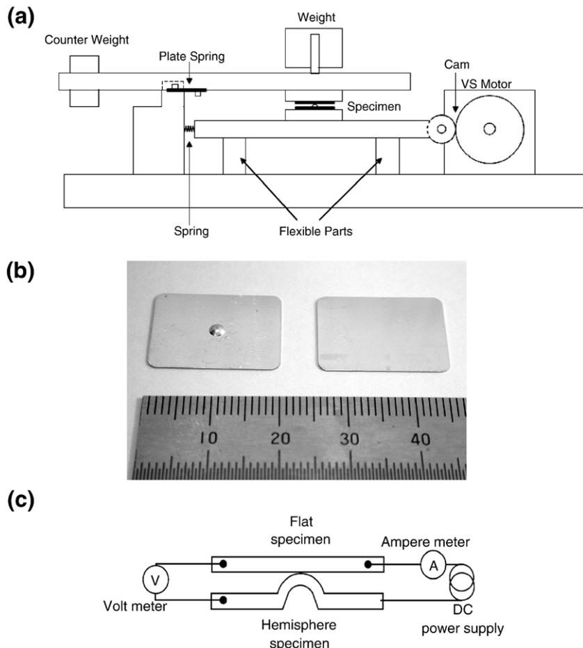
Fig. 1. (a) Schematic sketch of the fretting apparatus; (b) the rider and flat samples; (c) the geometry of the rider and flat samples and the circuit used to measure the contact resistance.
