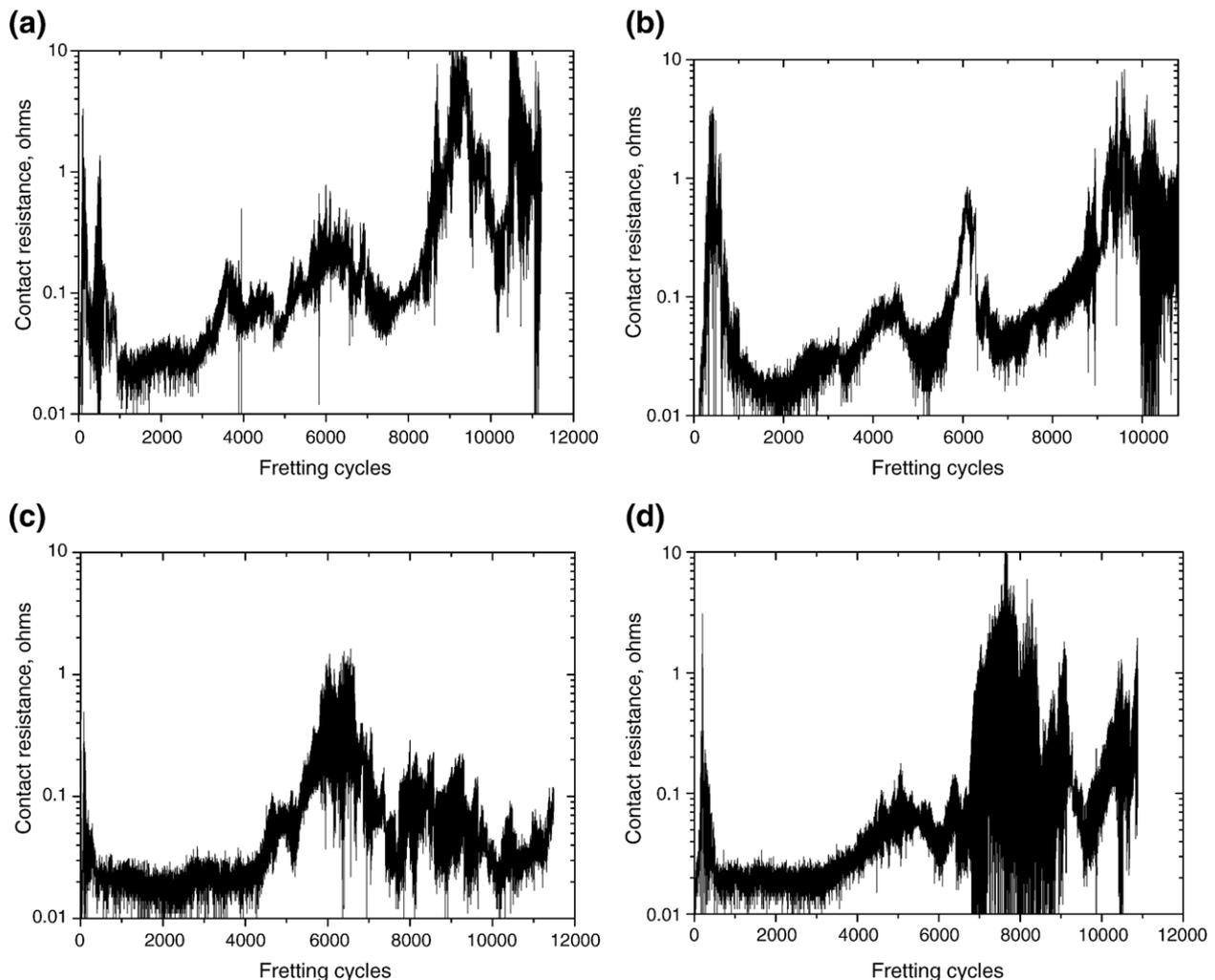
Fig. 2. Variation in contact resistance of the tin-plated brass contacts as a function of fretting cycles for a fretting frequency of 3 Hz at different normal loads (a) 0.25 N (b) 0.50 N (c) 1.0 N and (d) 1.5 N.
