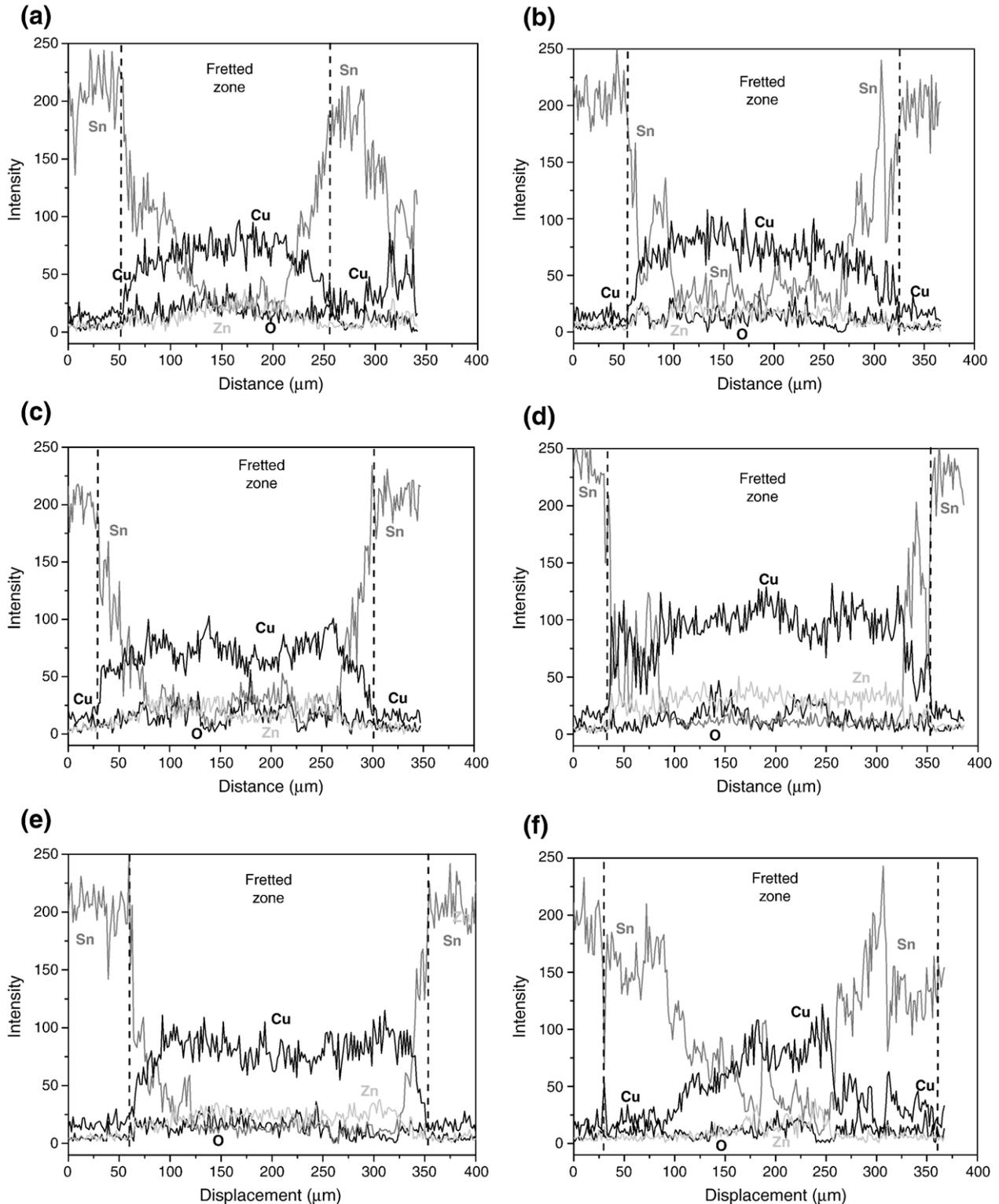
Fig. 10. EDX line scan performed across the fretted zone (indicated between dotted line) of the tin-plated brass contacts after 3600 fretting cycles obtained at various normal loads and fretting frequencies (a) 3 Hz, 0.25 N (b) 3 Hz, 0.50 N (c) 3 Hz, 1.0 N (d) 3 Hz, 1.5 N (e) 1 Hz, 1.0 N and (f) 8 Hz, 1.0 N.
