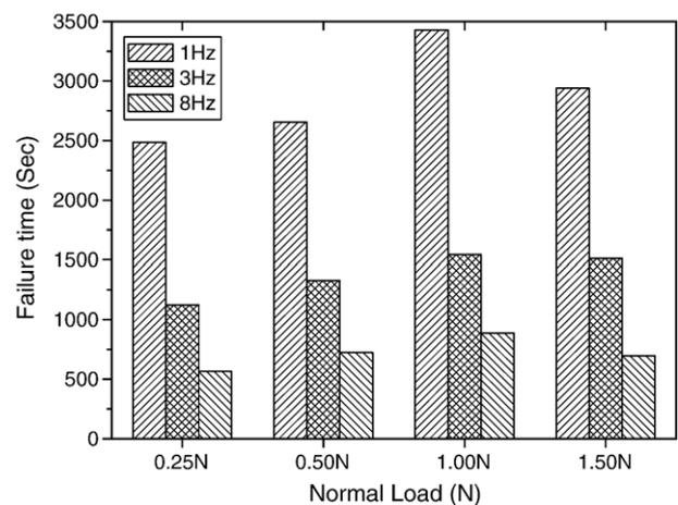
Fig. 4. Plot of failure time as a function of normal load and fretting frequency.
