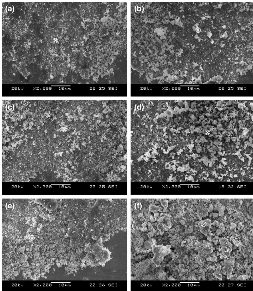
Fig. 9. Scanning electron micrograph of the wear debris and oxidation products present at the edge of fretted zone of tin-plated brass contacts after 3600 fretting cycles obtained at various normal loads and fretting frequencies (a) 3 Hz, 0.25 N (b) 3 Hz, 0.50 N (c) 3 Hz, 1.0 N (d) 3 Hz, 1.5 N (e) 1 Hz, 1.0 N and (f) 8 Hz, 1.0 N.
