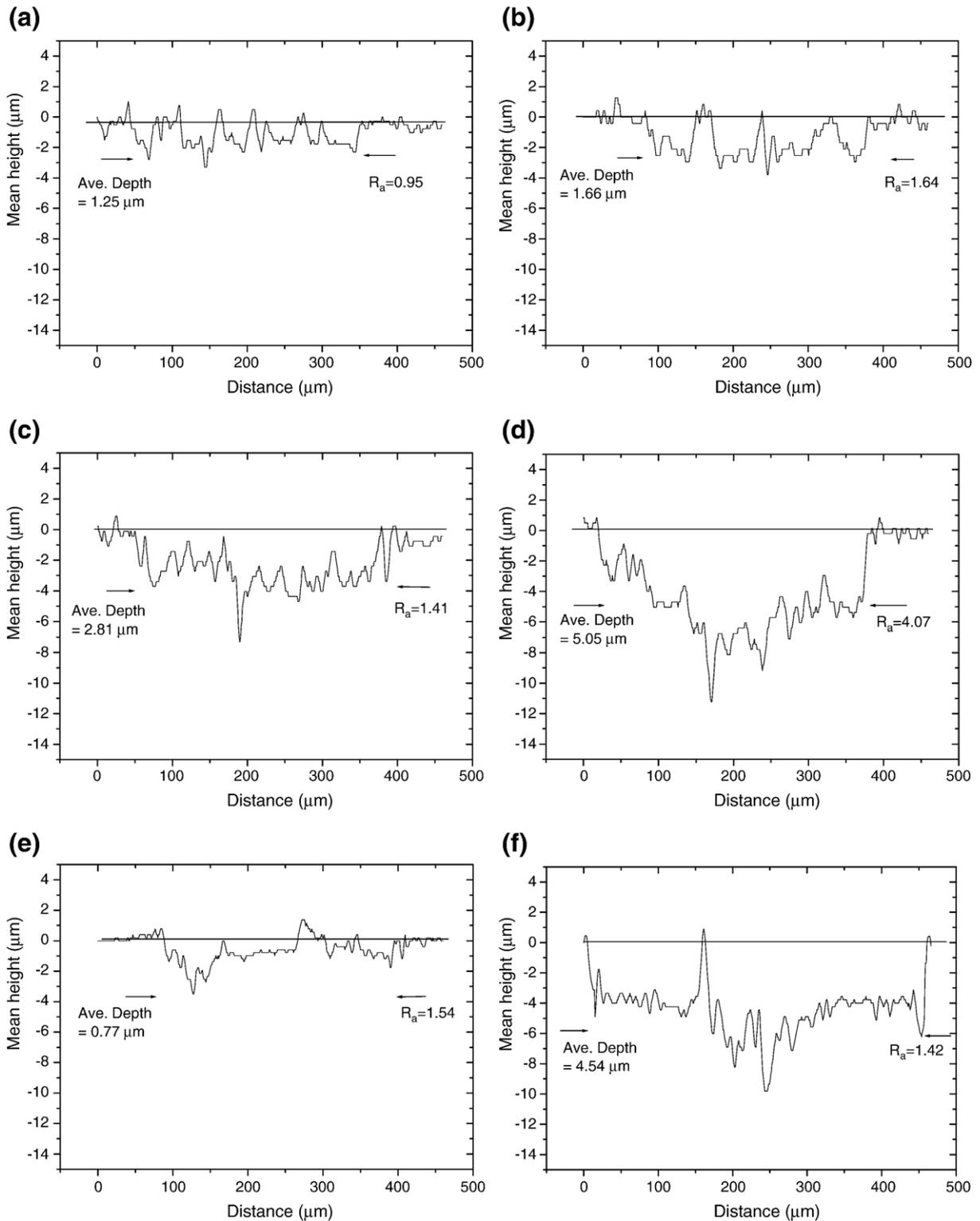
Fig. 5. Surface profile across the fretted zone of the tin-plated brass contacts after 3600 fretting cycles obtained at various normal loads and fretting frequencies. (a) 0.25 N, 3 Hz (b) 0.5 N, 3 Hz (c) 1.0 N, 3 Hz (d) 1.5 N, 3 Hz (e) 1 Hz, 1.0 N and (f) 8 Hz, 1.0 N.
