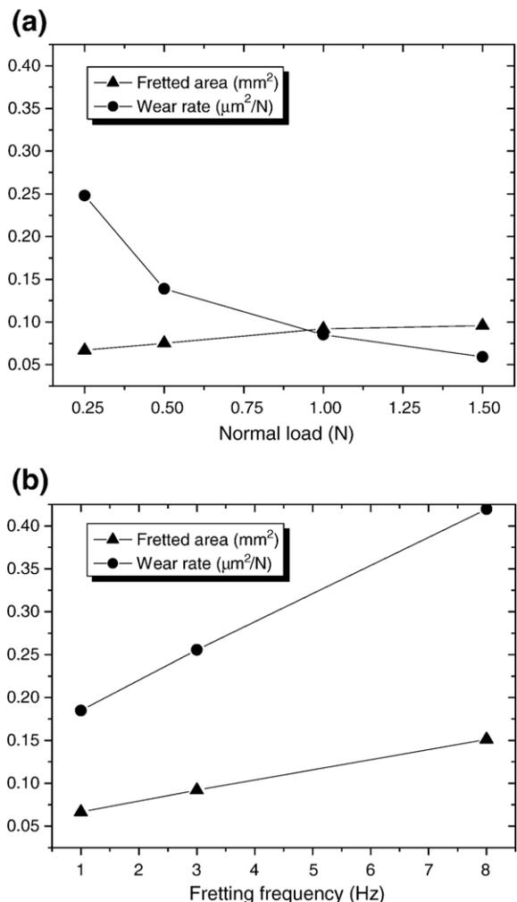
Fig. 7. Variation of fretted area and wear rate at 3600 fretting cycles as a function of (a) normal load at 3 Hz and (b) fretting frequency at 1 N load.
