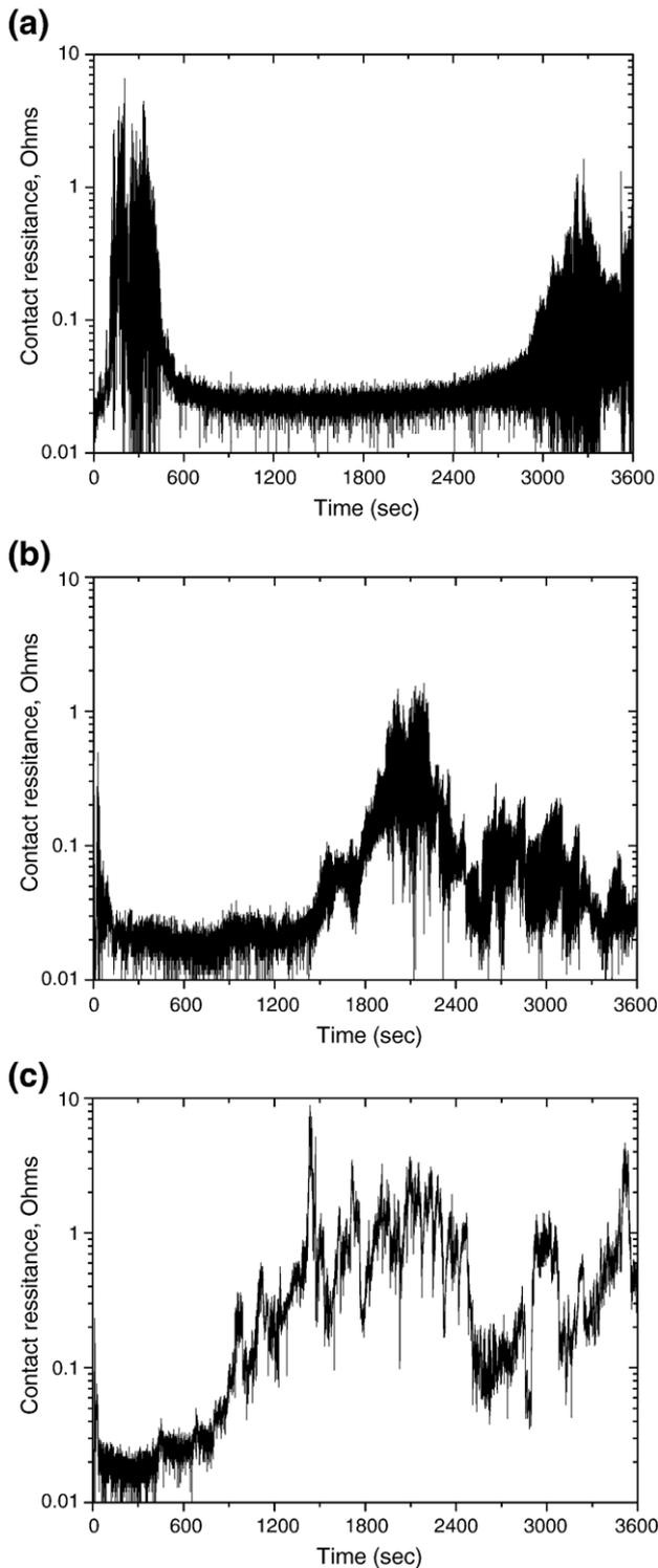
Fig. 3. Variation in contact resistance of the tin-plated brass contacts as a function of fretting time for a normal load of 1.0 N at different fretting frequencies (a) 1 Hz, (b) 3 Hz and (c) 8 Hz.
