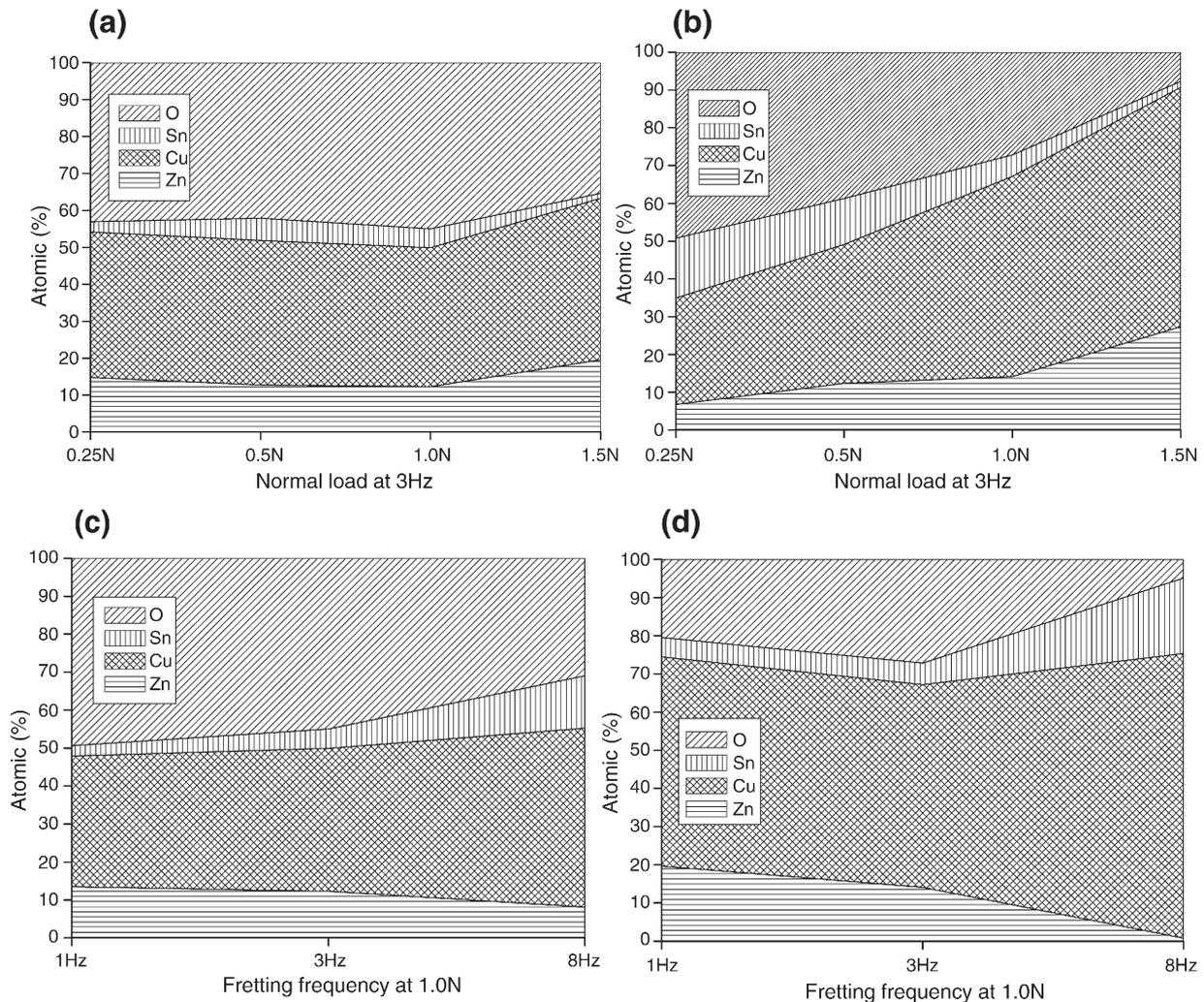
Fig. 11. Pictorial model depicting the variation in atomic concentration of zinc, copper, tin and oxygen of the oxide debris at the fretted zone with normal load variation at (a) center of fretted zone and (b) edge and with frequency variation at (c) center (d) edge.
