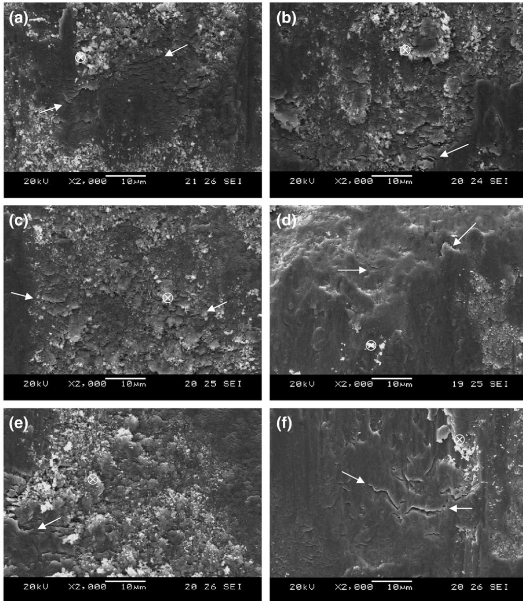
Fig. 8. Scanning electron micrograph of the worn out regions and oxide debris at the center of fretted zone of tin-plated brass contacts after 3600 fretting cycles obtained at various normal loads and fretting frequencies (a) 3 Hz, 0.25 N (b) 3 Hz, 0.50 N (c) 3 Hz, 1.0 N (d) 3 Hz, 1.5 N (e) 1 Hz, 1.0 N and (f) 8 Hz, 1.0 N.
