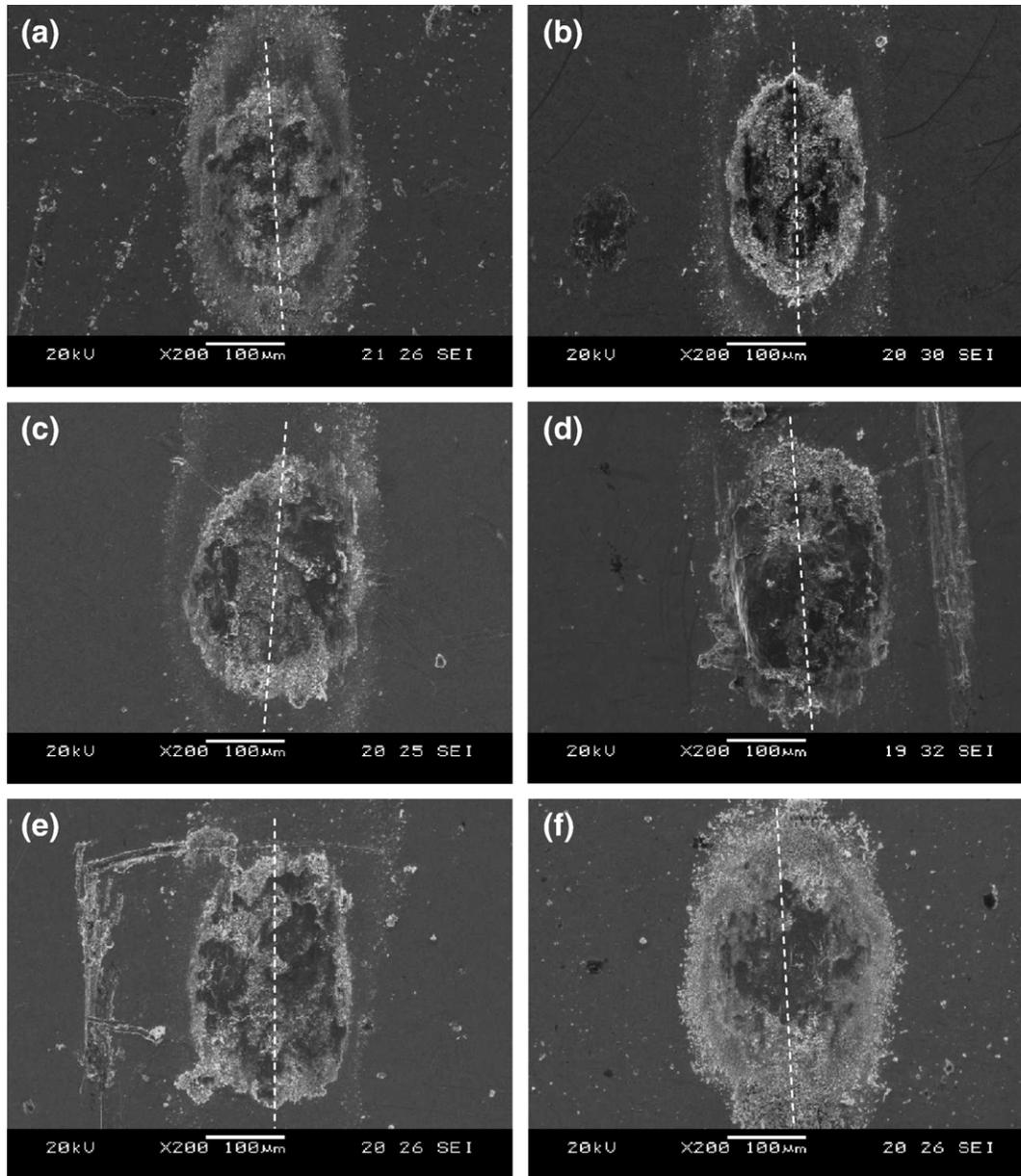
Fig. 6. Surface morphology of the fretted tin-plated brass contacts after 3600 fretting cycles obtained at various normal loads and fretting frequencies (a) 0.25 N, 3 Hz (b) 0.5 N, 3 Hz (c) 1.0 N, 3 Hz (d) 1.5 N, 3 Hz (e) 1 Hz, 1.0 N and (f) 8 Hz, 1.0 N.
