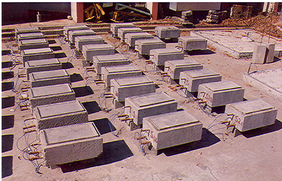
Fig. 2. Concrete specimens under exposure conditions in exposure yard.
