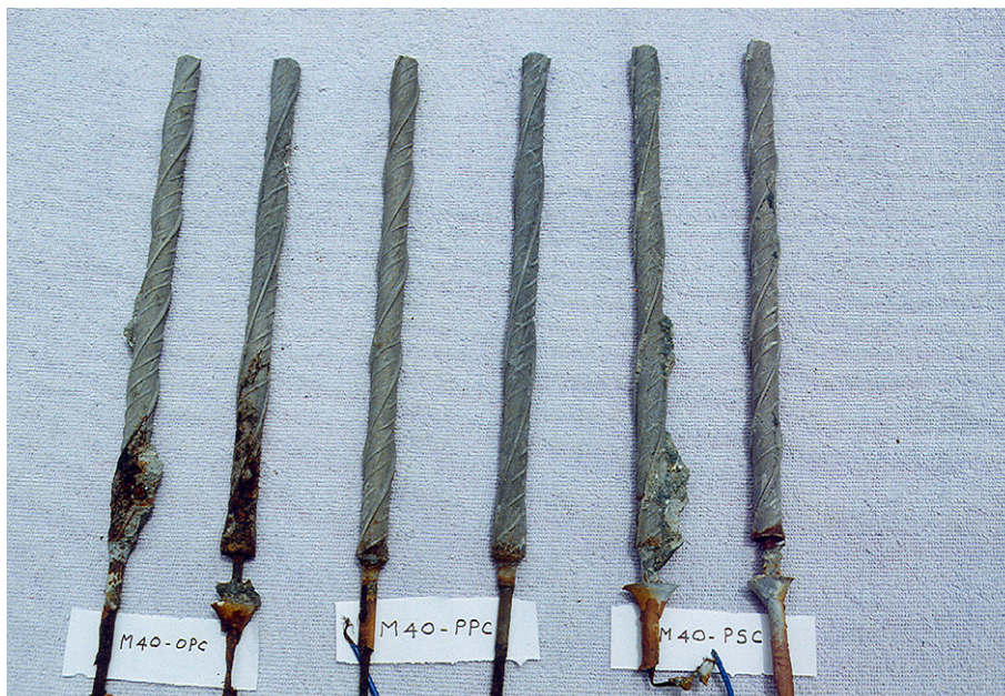
Fig. 11. Extent of rust on rebars embedded in 40 MPa concrete.
