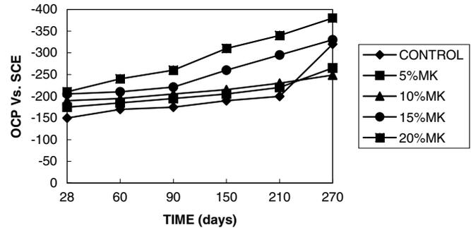
Fig. 2. Potential time behaviour of carbon steel embedded in concrete with MK.
