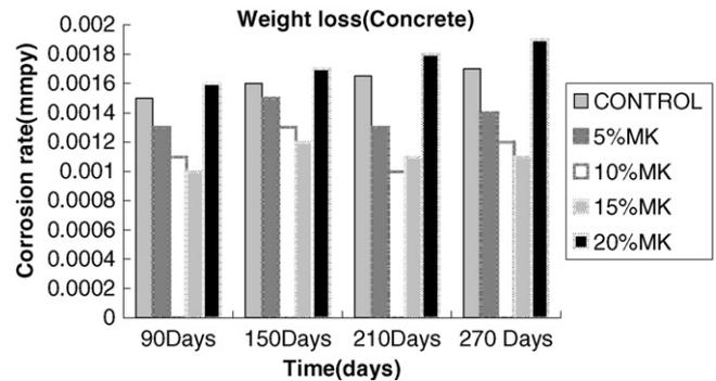
Fig. 4. Weight loss measurement for concrete specimens with MK.
