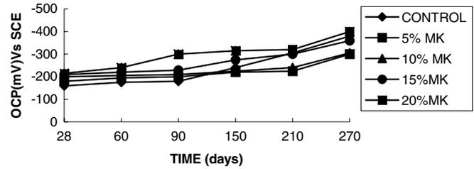
Fig. 1. Potential time behaviour of carbon steel embedded in mortar with MK.
