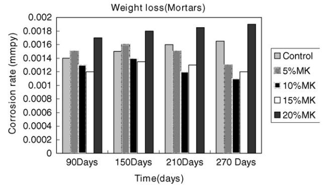
Fig. 3. Weight loss measurement for mortar specimens with MK.
