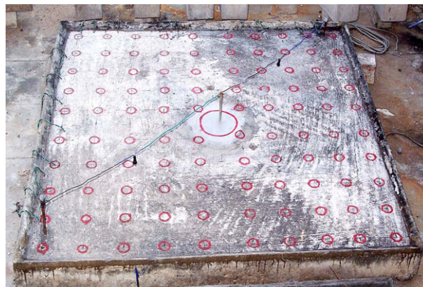
Fig. 1. Cathodically protected chloride contaminated concrete slab with magnesium alloy anode plugged at the center.
