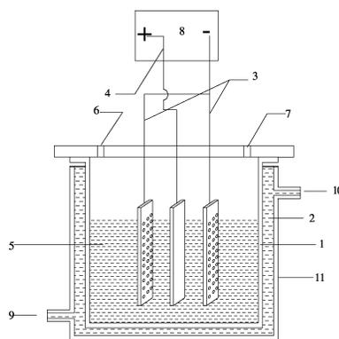
**Figure 1.** Laboratory scale cell assembly. Legend: 1, cell; 2, thermostatic water; 3, stainless steel cathode; 4, anode; 5, electrolyte; 6 and 7, holes to introduce the pH sensor and thermometer; 8, DC source; 9, inlet; 10, outlet; and 11, thermostat.
