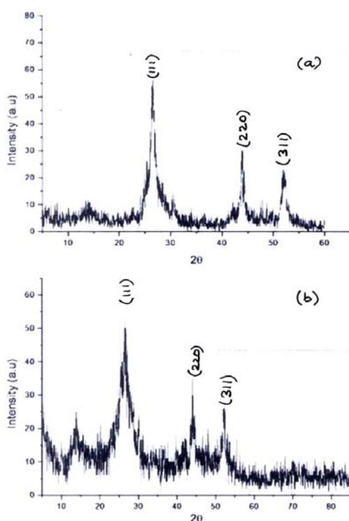
Fig.1 - XRD patterns of CdS films deposited at different deposition current densities (a)  $50 \text{ mA cm}^{-2}$  (b)  $300 \text{ mA cm}^{-2}$
