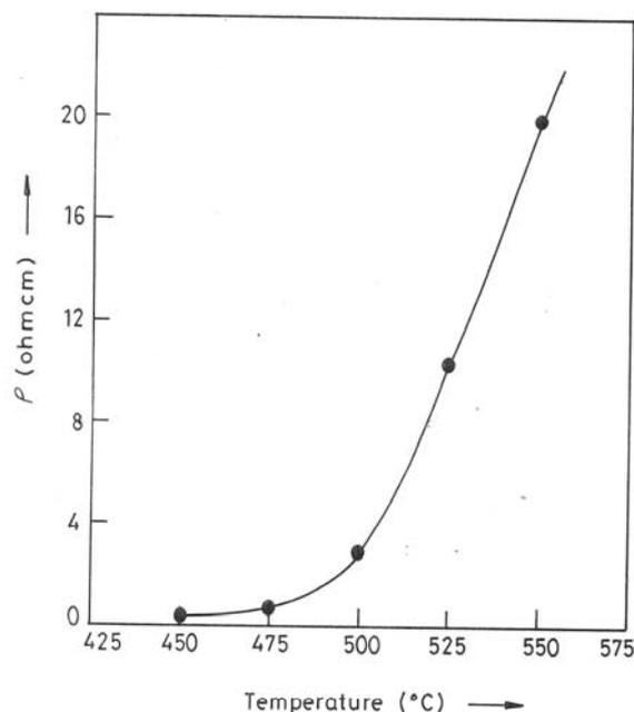
Fig.6. Variation of resistivity of CdS films with post annealing temperature
