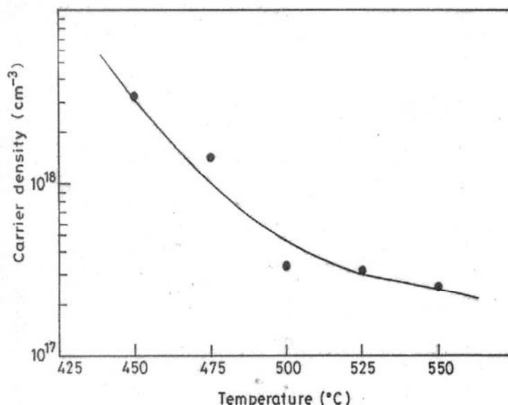
Fig.8. Variation of Carrier density of CdS films with post annealing Temperature.
