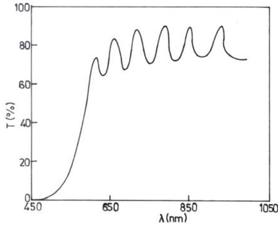
Fig.4. Transmission spectra of CdS films deposited at 300 mA cm<sup>-2</sup>
