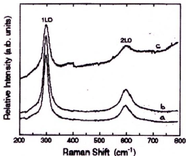
Fig.9. Laser Raman Spectra of CdS films deposited at different deposition current densities (a)  $50 \text{ mA cm}^{-2}$  (b)  $150 \text{ mA cm}^{-2}$  (c)  $300 \text{ mA cm}^{-2}$
