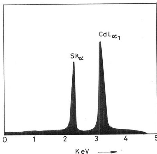
Fig.3. EDAX spectrum of CdS films heated at 550 °C
