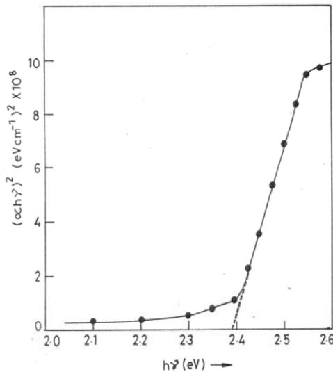
Fig. 5.  $(\alpha h\nu)^2$  vs  $h\nu$  plot of the CdS films annealed at 550 °C
