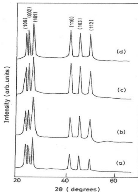
Fig. 2 - XRD patterns of CdS films annealed in argon atmosphere at different temperatures (a) 450°C (b) 500°C (c) 525°C (d) 550°C.
