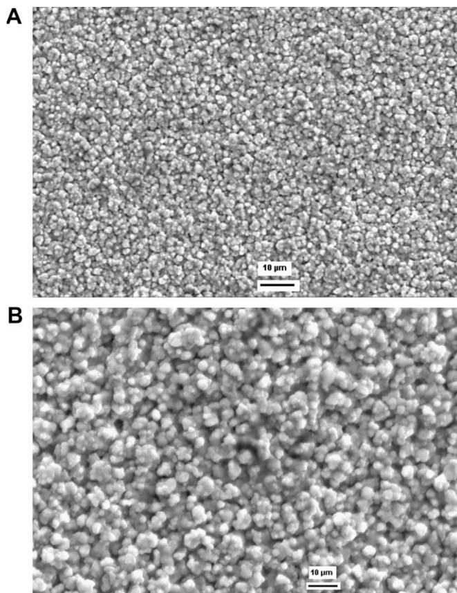
**Fig. 2.** (A and B) SEM surface morphology of PE-deposited chromium at an average current density was 10.4 A/dm<sup>2</sup> and 20 A/dm<sup>2</sup> from Cr(III) and Cr(VI)-baths in 30 min.
