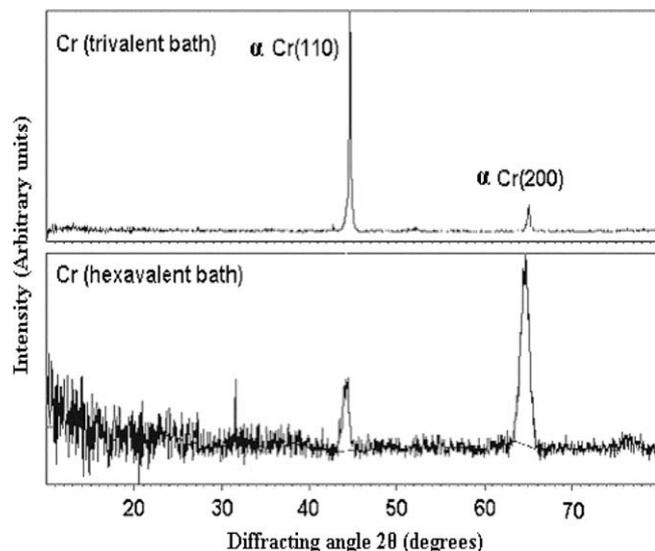
**Fig. 3.** XRD pattern of chromium coatings from Cr(III) and Cr(VI)-baths.
