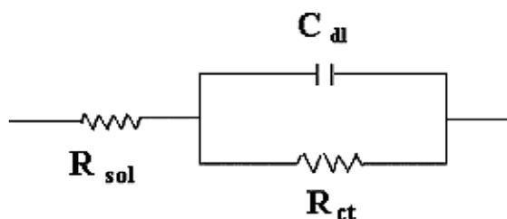
Fig. 6. Equivalent circuit diagram of impedance spectra for electrodeposited chromium in 3.5%NaCl electrolyte.
