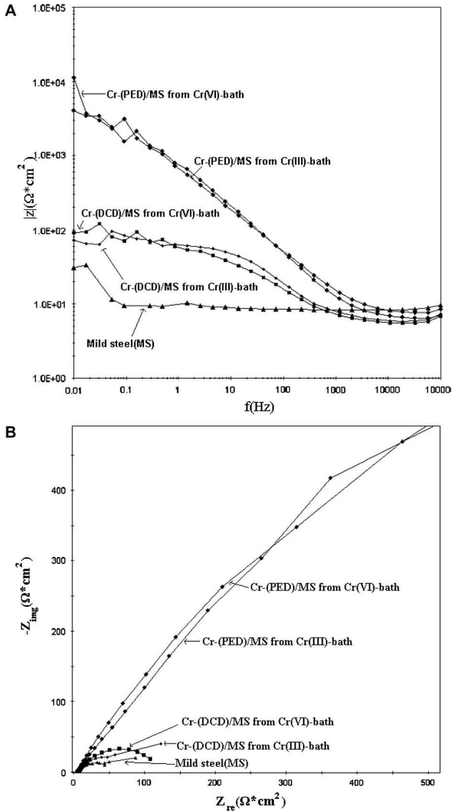
Fig. 5. Impedance spectra of MS panel, Cr on MS (DCD) and Cr on MS (PED) from Cr(III) and Cr(VI)-baths: (A) Bode–Bode plot; (B) Nyquist plot.
