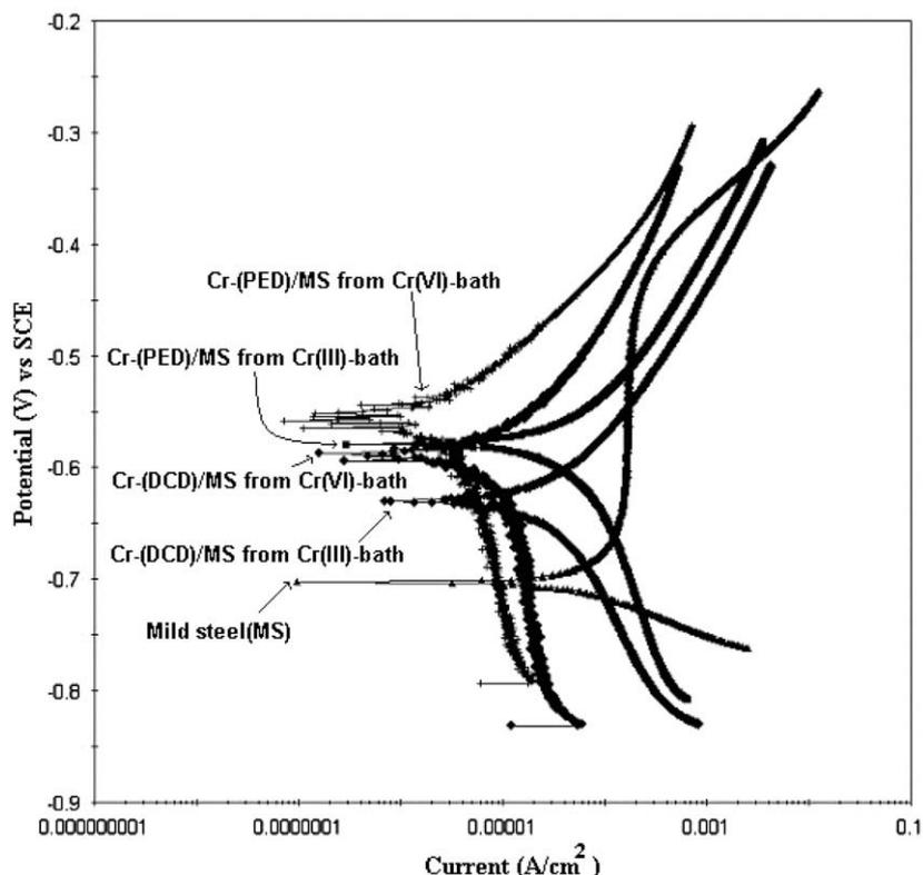
Fig. 4. Polarization studies of MS panel, Cr on MS (DCD) and Cr on MS (PED) from Cr(III) and Cr(VI)-baths in 3.5% w/v NaCl electrolyte.
