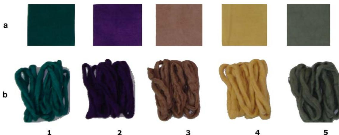
**Fig. 5** Photograph of dyed samples **a** fabric and **b** yarn with different vat dyes 1. Green FFB, 2. Violet RR, 3. Brown BR, 4. Yellow RT, and 5. Olive R under optimized experimental conditions
