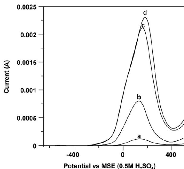
Fig. 5. Linear sweep voltammetric response of various compositions of Au-Pt/C in 0.5 M H<sub>2</sub>SO<sub>4</sub> containing 0.1 M methanol at scan rate 0.005 V s<sup>-1</sup>: (a) (30:10); (b) (20:20); (c) (10:30); (d) (0:40).
