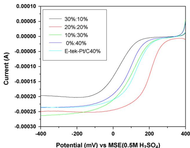
Fig. 4. Linear sweep voltammograms recorded in O<sub>2</sub>-saturated 0.5 M H<sub>2</sub>SO<sub>4</sub> solution at 900 rpm for Au–Pt/C bimetallic nanoparticles: ( ) (30:10); ( ) (20:20); ( ) (10:30); ( ) (0:40); ( ) (E-tek-Pt/C 40) scan rate = 0.005 V s<sup>-1</sup>.
