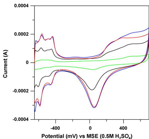
Fig. 3. Cyclic voltammograms of Au–Pt/C bimetallic nanoparticles recorded in 0.5 M H<sub>2</sub>SO<sub>4</sub> solution at a scan rate of 0.05 V s<sup>-1</sup>: ( ) (0:40), ( ) (10:30), ( ) (20:20), ( ) (30:10).
