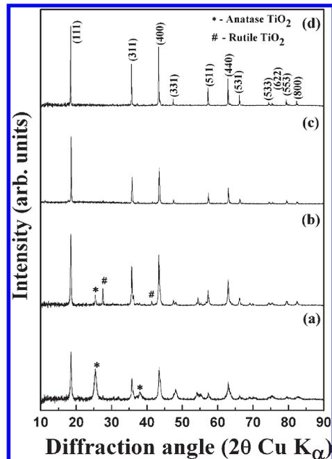
**Figure 2.** Powder XRD patterns for the products formed by the combustion of lithium and titanium nitrates with glycine at (a) 500 °C, (b) 700 °C, (c) 800 °C, and (d)  $\text{Li}_4\text{Ti}_5\text{O}_{12}$  prepared by solid-state method.
