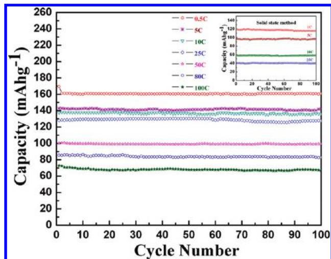
**Figure 7.** Capacity versus cycle number plot for nanocrystalline  $\text{Li}_4\text{Ti}_5\text{O}_{12}$  synthesized by the combustion method at different discharge rates. Inset shows capacity versus cycle number for bulk  $\text{Li}_4\text{Ti}_5\text{O}_{12}$ .
