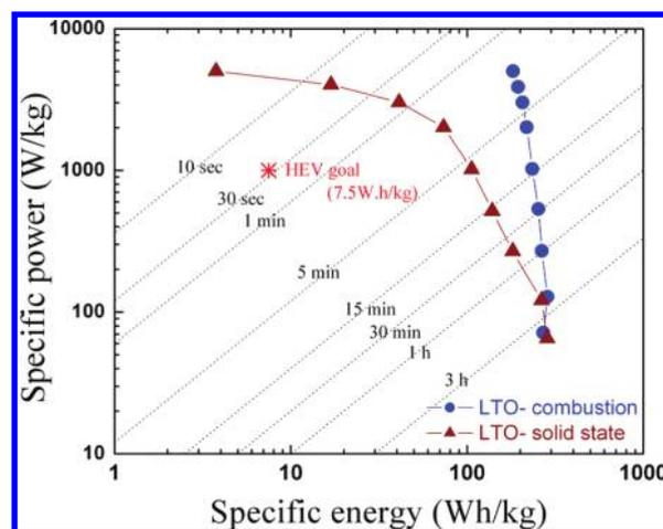
**Figure 8.** Ragone plot comparing the performance of  $\text{Li}_4\text{Ti}_5\text{O}_{12}$  prepared by (-●-) combustion method and (-▲-) solid-state method when paired with metallic lithium; (\*) DOE benchmark for HEVs.
