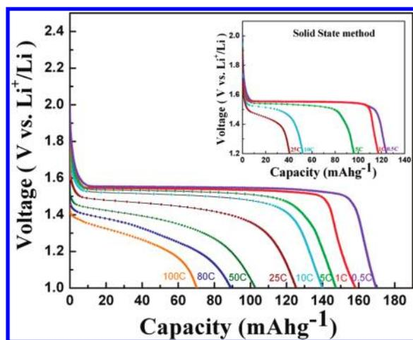
**Figure 6.** Capacity-voltage profile for nanocrystalline  $\text{Li}_4\text{Ti}_5\text{O}_{12}$  synthesized by the combustion method at different rates. Inset shows capacity voltage profile for bulk  $\text{Li}_4\text{Ti}_5\text{O}_{12}$  prepared by the solid-state method.
