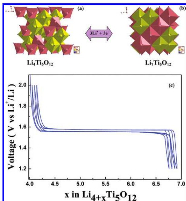
**Figure 5.** Structure of (a) spinel  $\text{Li}_4\text{Ti}_5\text{O}_{12}$  and (b) ordered rocksalt-phase  $\text{Li}_7\text{Ti}_5\text{O}_{12}$ ; (c) voltage-composition curves showing the electrochemical transformation of  $\text{Li}_4\text{Ti}_5\text{O}_{12}$ – $\text{Li}_7\text{Ti}_5\text{O}_{12}$  during galvanostatic charge–discharge cycles at C/2 rate at 30 °C.
