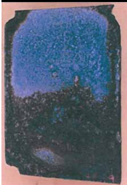
GI panel exposed at Kochi Naval Base over a period of 1.5 years.
