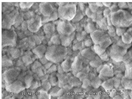
8 Image (SEM) of electroless Ag deposited at 60°C and pH 10.8 for 30 min
