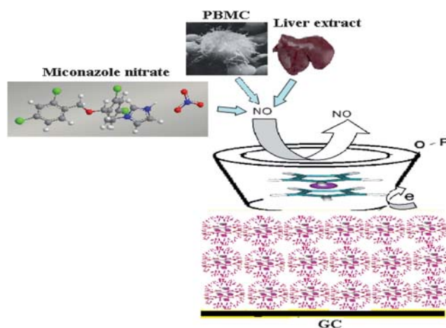
Scheme 1 Schematic diagram depicting the soluble cyclodextrin encapsulated ferrocene mediating the reduction of NO to \text{NO}^- for the assay of NO in few biological systems.
