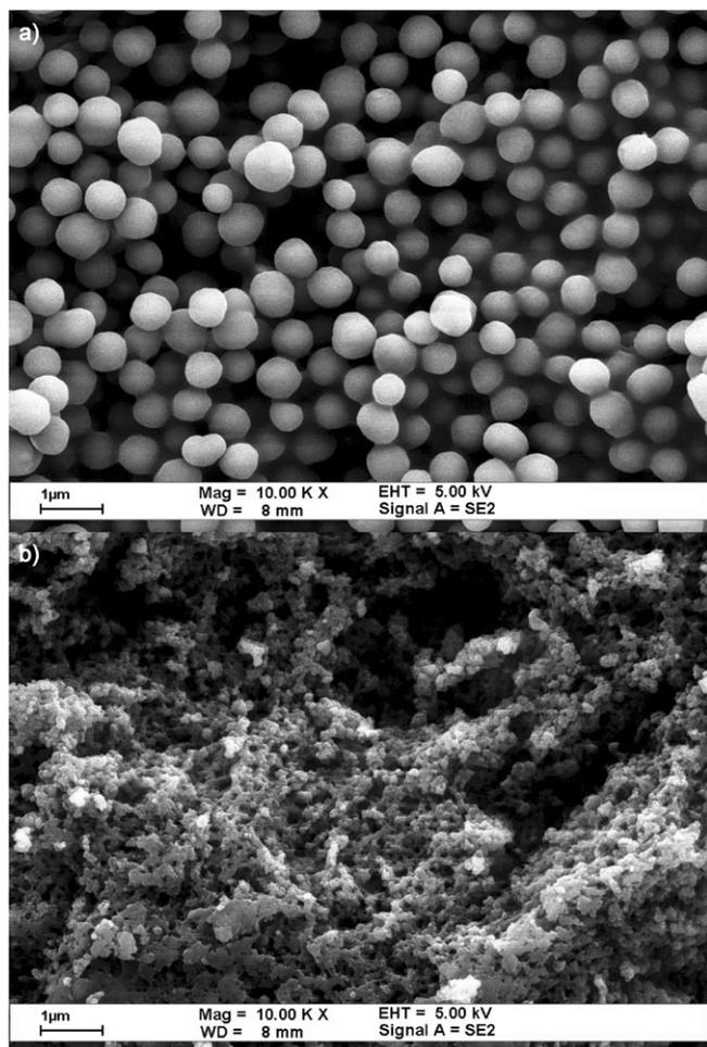
Fig. 2. The morphologies of MIP particles prepared by (a) precipitation polymerization, (b) traditional bulk polymerization [15].
