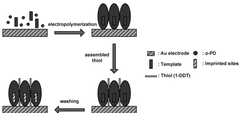
Fig. 3. Schematic representation of the imprinting modification of *o*-PD on the gold surface by 1-DDT.
