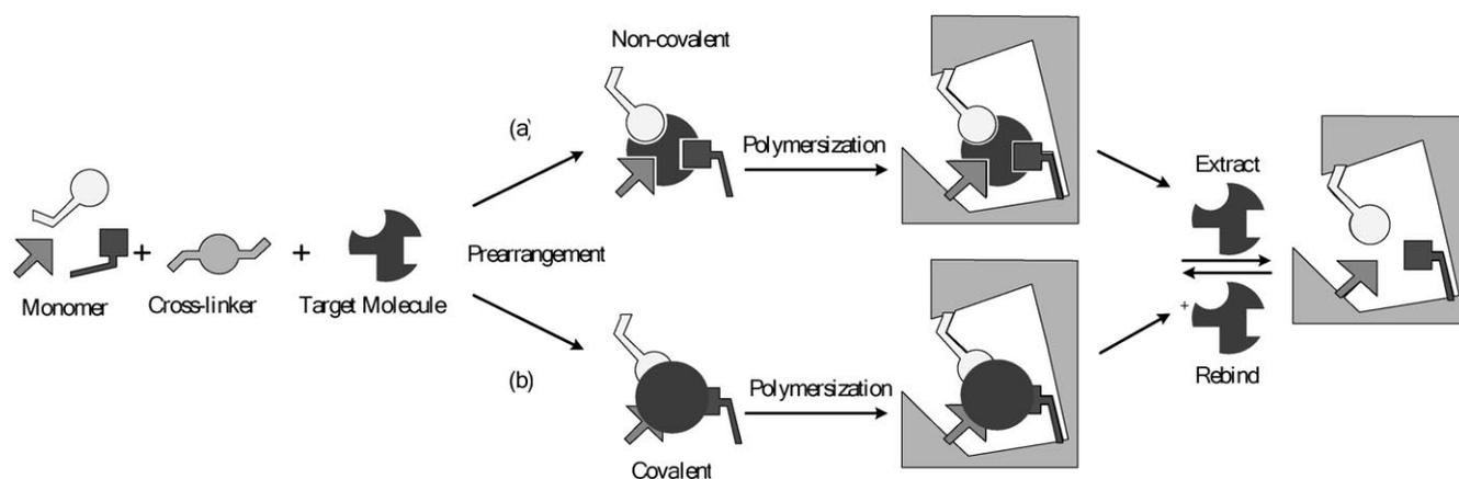
Fig. 1. Schematic overview of molecular imprinting technique; (a) and (b) shows the pathway for noncovalent and covalent imprinting.
