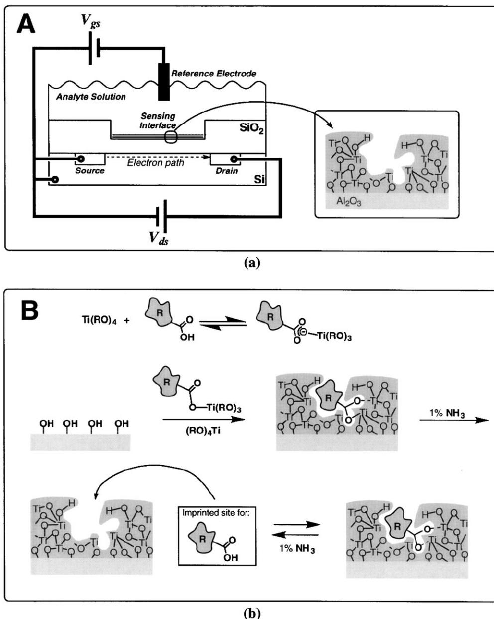
Fig. 5. (a) Schematic configuration of molecular imprinted ISFET device. (b) Preparation of the MIP on  $\text{TiO}_2$  thin film acting as a sensing interface on the ISFET gate (reproduced from [78]).
