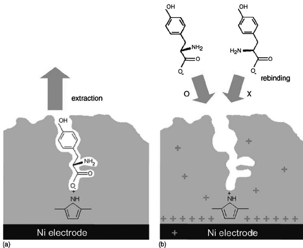
Fig. 6. Schematic diagram of (a) the extraction of template from a D-tyrosine imprinted polypyrrole film and (b) the rebinding of D-tyrosine induced by a positive potential (reproduced from [52]).
