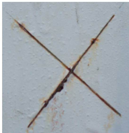
Fig. 9. Photograph of tungstate doped PANI incorporated paint coated with top coated panels exposed to salt spray.
