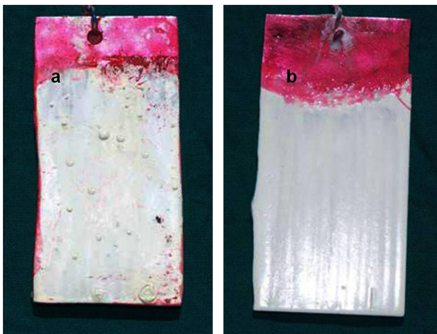
Fig. 6. Photograph of AA 7075 alloy after exposure to salt spray for 4 weeks. (a) Epoxy coated sample; (b) Electropolymerised PANI with epoxy coating.
