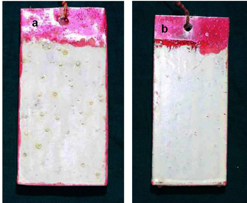
Fig. 3. Photograph of AA 2024 alloy after exposure to salt spray for 4 weeks. (a) Epoxy coated sample; (b) electropolymerised PANI with epoxy coating.
