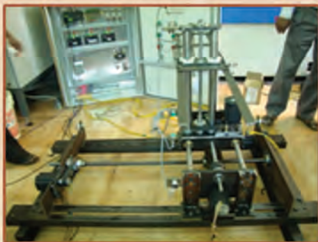
Three axes Prototype profile polishing machine
