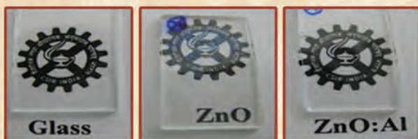
Photograph of bare glass and, ZnO and ZnO:Al coated glass plates revealing the transparent nature of the films.
