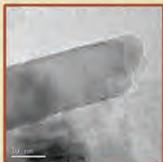
The TEM images and electron diffraction of CoO nanowires at various magnifications
