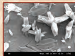
(a) through (g). Calcareous deposition on cathodic stainless steel surfaces. The images (a), (c) and (e) show deposits formed at night, while (b), (d) and (f) are corresponding images for daytime.
