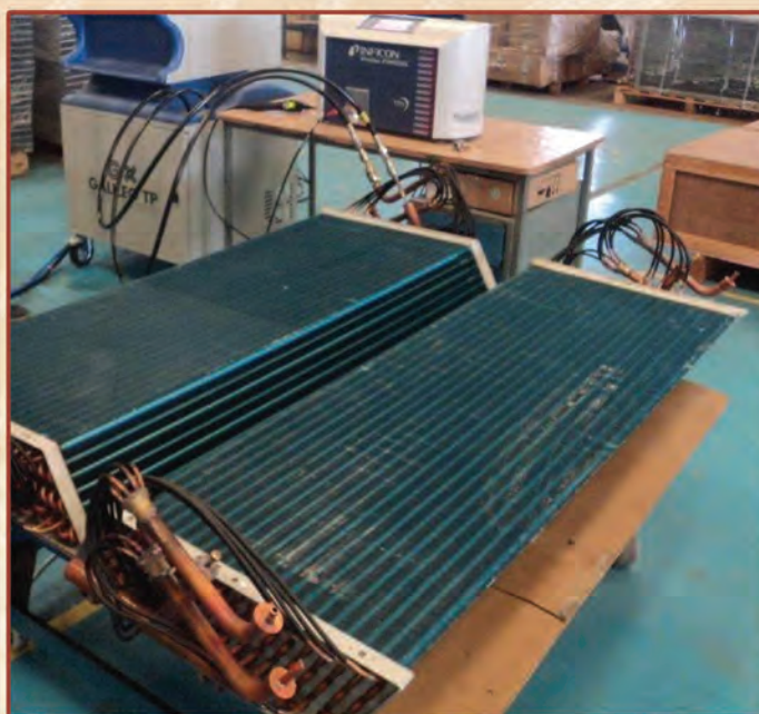
Metro Rail Cooling system: Testing of brazed joints on Copper tubes
