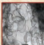
Left: A SEM image of kish graphite showing characteristic flaky morphology.
