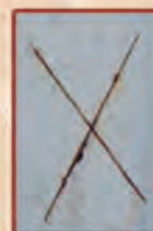
Photograph of tungstate doped PANI incorporated paint coated panels exposed to Salt spray
