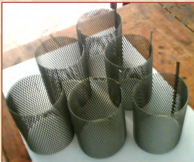
Design, fabrication and processing of cylindrical mixed metal oxide coated titanium expanded mesh anodes for concrete corrosion studies (CECRI)
