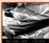
Left: A SEM image of kish graphite showing characteristic flaky morphology.
