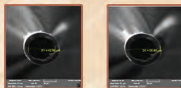
SEM image of the micropipette with inner diameter 42.56 \mu\text{m} and outer diameter 56.88 \mu\text{m} this is filled with an aqueous solution.
