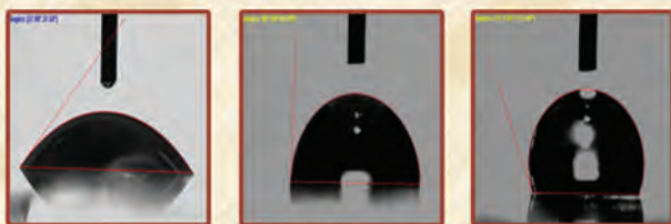
Images showing the increase in water contact angle (WCA) over glass, ZnO and ZnO:Ti coated glass.
