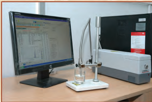
PARTICLE SIZE ANALYZER – MICROTRAC
