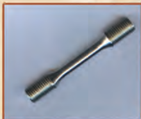
Creep Testing Specimen
