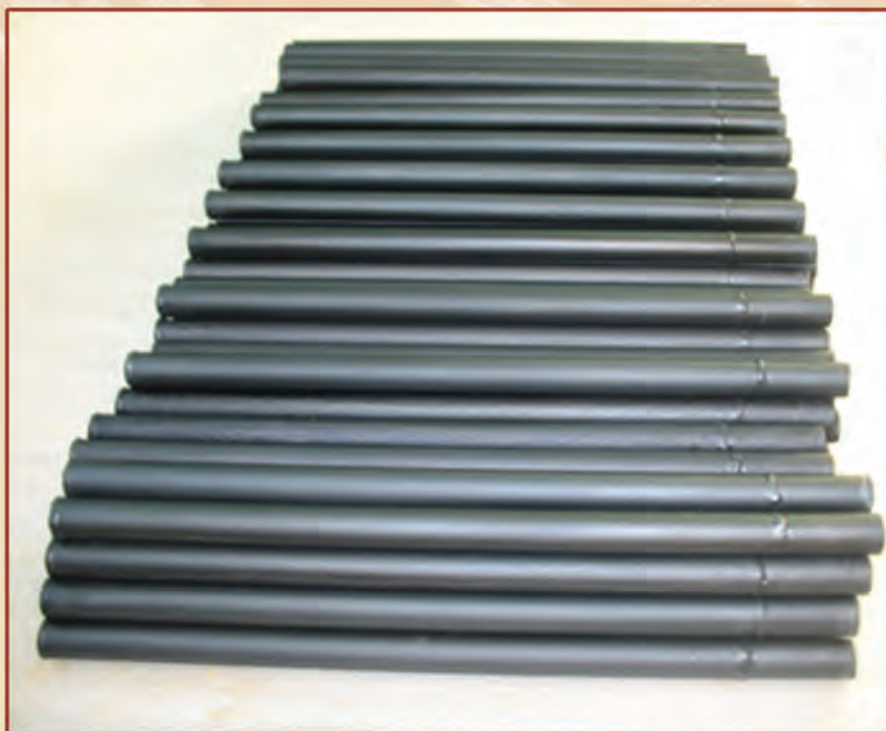
Design, fabrication and processing of MMO coated tubular anodes for cathode protection
