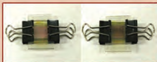
ZnO/dye electrode Counter electrode
