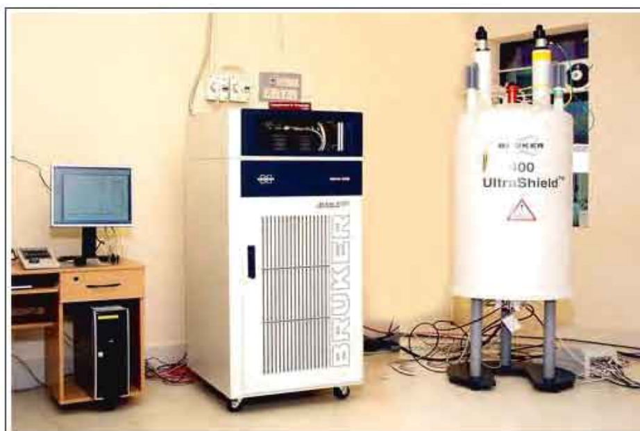
NMR spectrometer Advance 400 MHz (Bruker)
