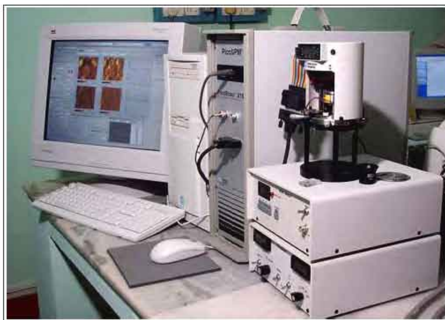
Scanning Probe Microscope (SPM) PicaSPM Picascan 2100 (Molecular Imaging)
