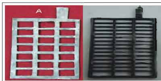
Lead alloy grid with punched design (left) and Lead-coated plastic grid with dove tail design (right)
