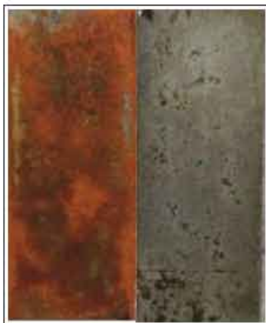
Images of MS coupons in natural seawater (left) without and (right) with inhibitor (260 ppm) after 18 days exposure.
