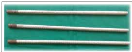
Nickel-coated rebars for macro cell test.
