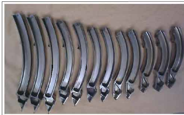
Heat-treated, polished and chromated slot track components
