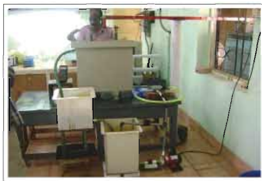
Purification of recycled base (impure TMAH) in 500 ampere rating electrolyser.
