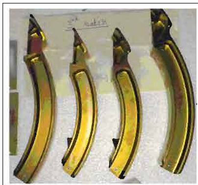
Heat-treated slot track components
