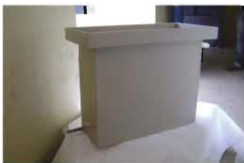
Electrolyser for treatment of impure TMAH to TMAChloride fabricated from polystone
