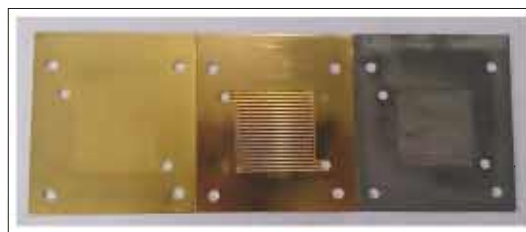
Coated SS plates: TiN; gold; and plasma nitride.
