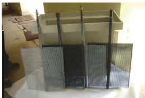
500A electrolyser with anodes and cathodes for purification of recycled base to TMAH
