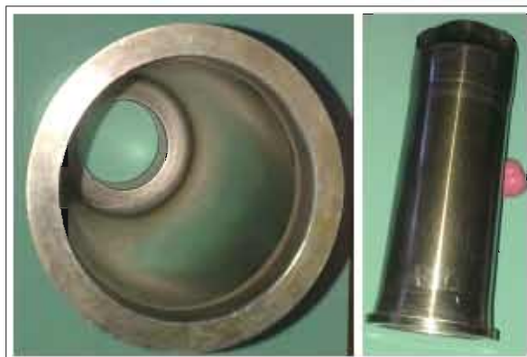
Electroless nickel-plated, heat-treated, polished and chromated forward cylinder and rod impulse
