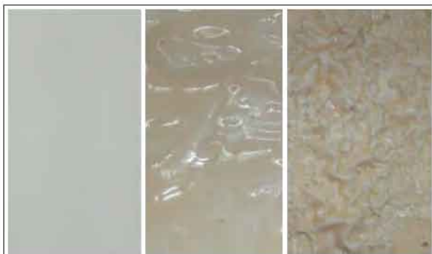
ZRP + epoxy paint coated panel (left); neutral paint remover applied on surface (middle); coating lifted from the surface after 30 min (right).
