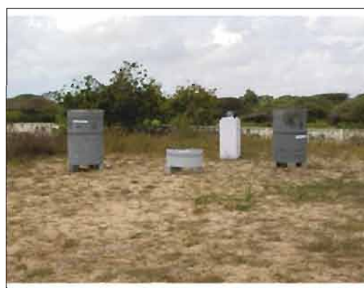
Canister bulk head exposed to marine environment at Mandapam yard to compare the life from actual field conditions with laboratory-simulated conditions.
