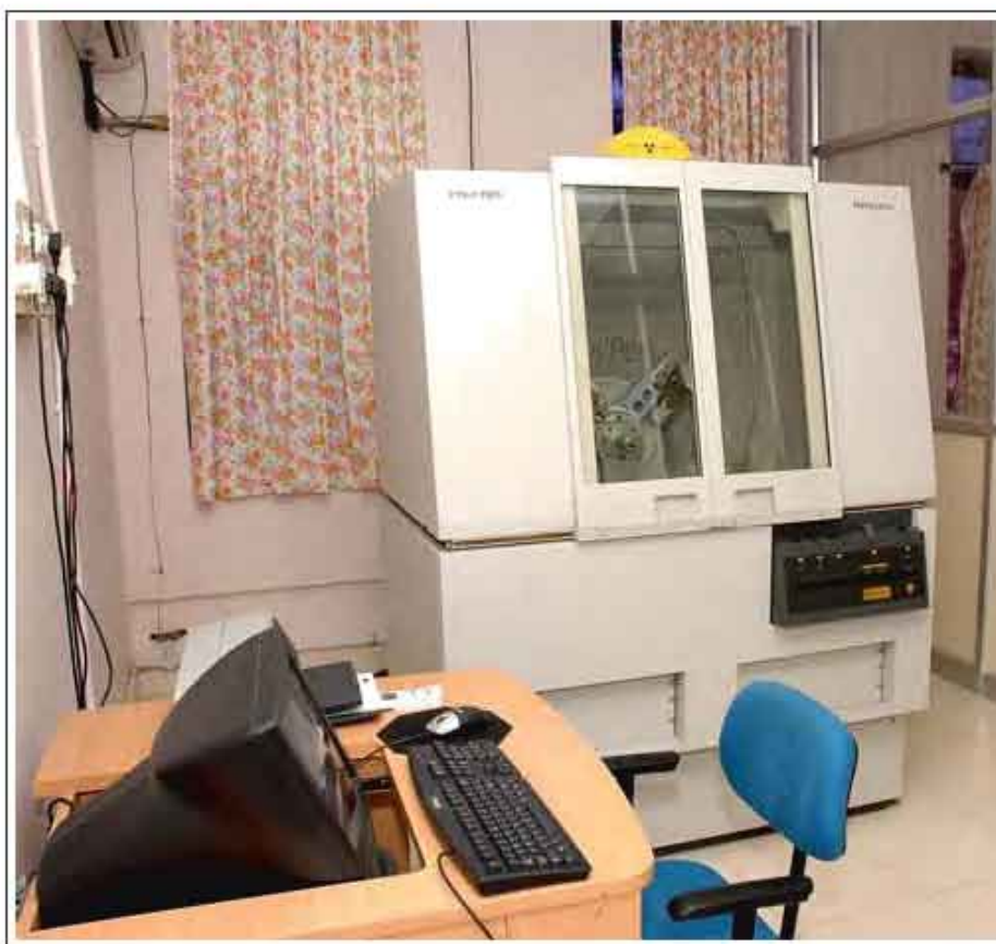
Powder X-ray Diffractometer (XRD) PW3040/60 X'pert PRO (PANalytical)
