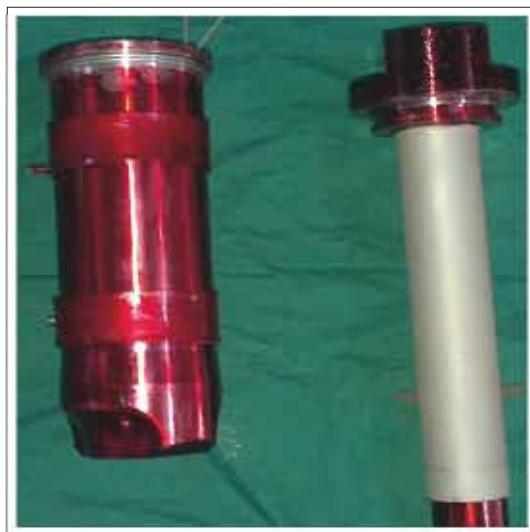
Electroless nickel-plated forward cylinder and rod impulse
