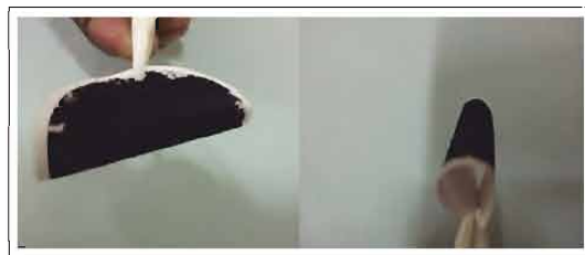
Flexible graphene-PDMA film on membrane filter PTFE.
