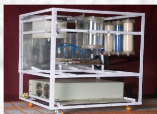
PEM electrolyzer for hydrogen generation
