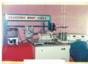
Electrochemical Flow Cell for the conversion of L-Cystine to L-Cysteine
