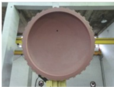
Lid of Hydroclave coated with CECRI developed coating at VSSC, Thiruvananthapuram, Technology transferred to VSSC, Thiruvananthapuram
