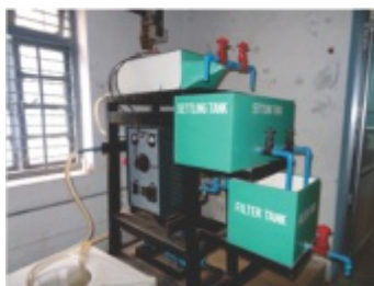
200 l/h Electrochemical defluoridation unit
