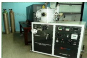
KrF based Pulsed Laser Deposition facility at CECRI
