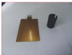
Colored stainless steel panels and tubes
