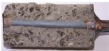
Corrosion free rebar after time to cracking study
