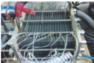
20 cell, 1 kW PEMFC stack H_2 - O_2 ; 1.45 kW; H_2 -air: 1.0 kW
