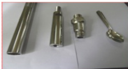
Electropolished stainless steel piston rods and other components
