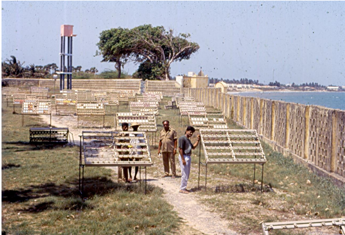
Atmospheric Corrosion Testing Yard on the shore of Gulf of Mannar, Bay of Bengal
