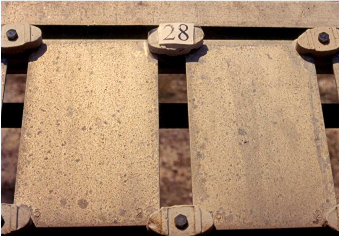
Aluminium alloy of Institute of Metallurgy, Russia exposed at Mandapam for 20 years
