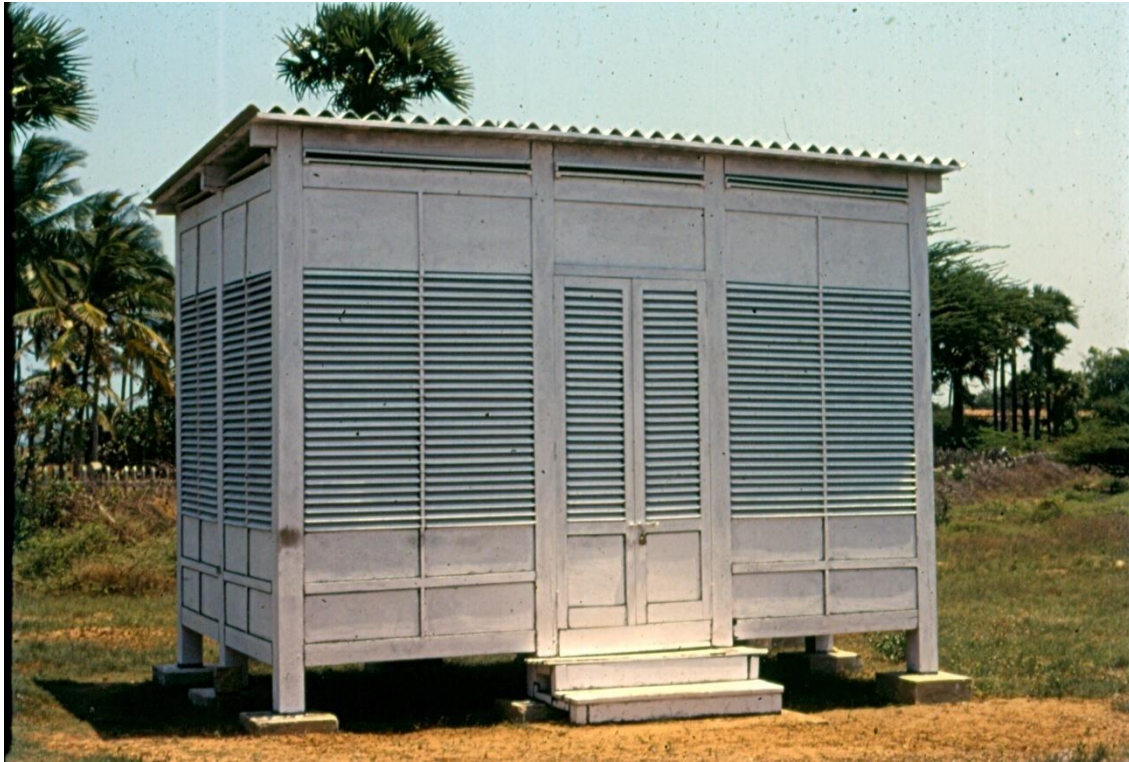
Stevenson chamber for indoor evaluation of materials
