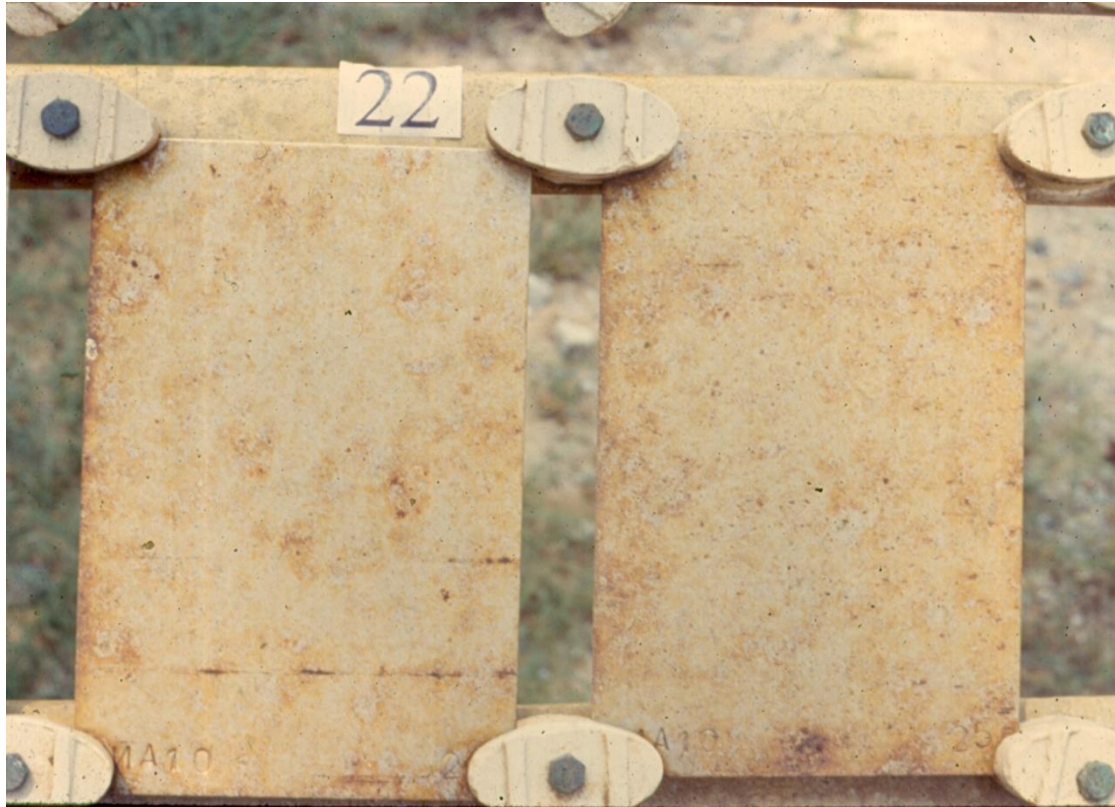
Austenitic Stainless steel of Institute of Metallurgy, Russia exposed at Mandapam for 20 years
