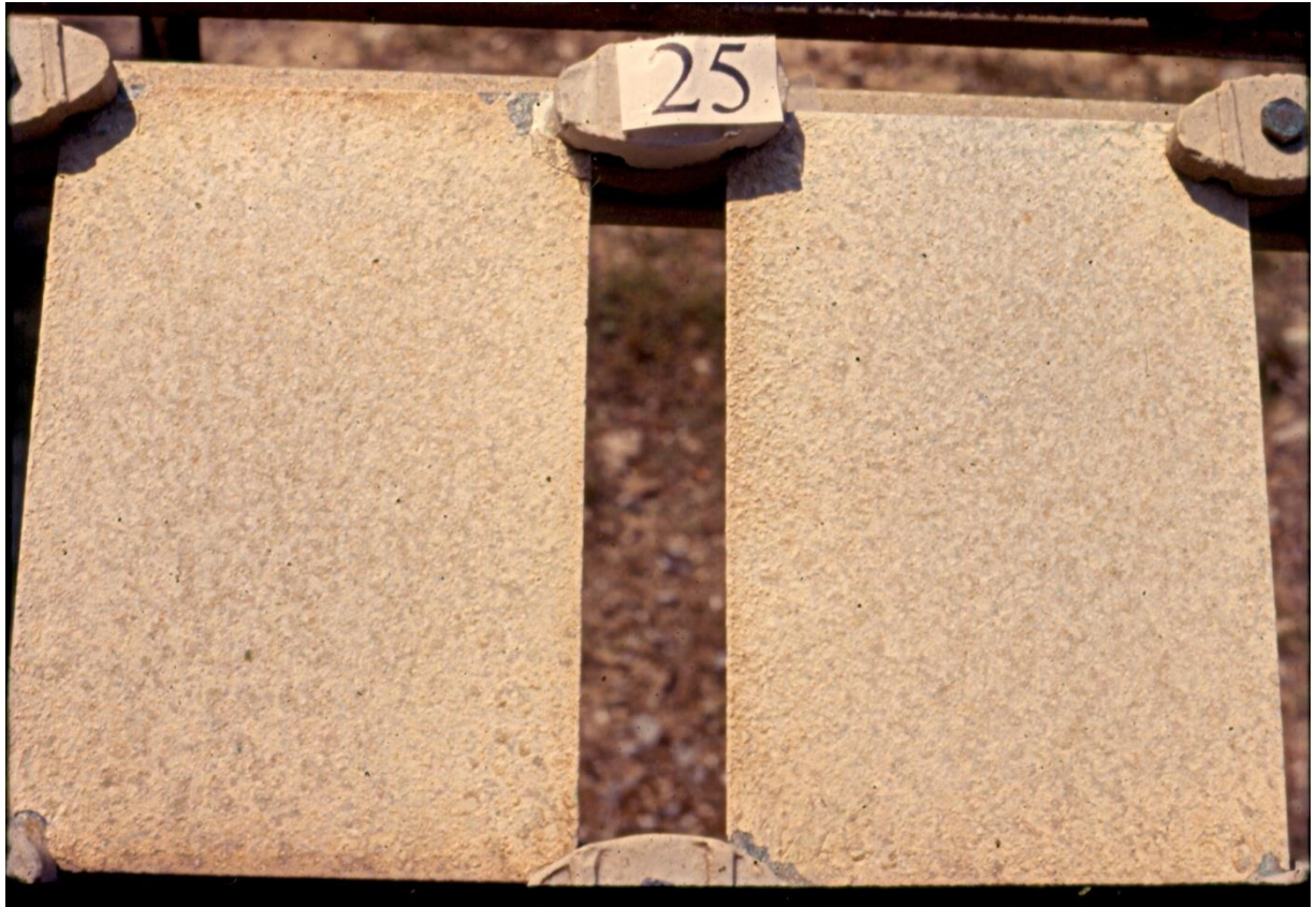
Dezincified Brass of Institute of Metallurgy, Russia exposed at Mandapam for 20 years
