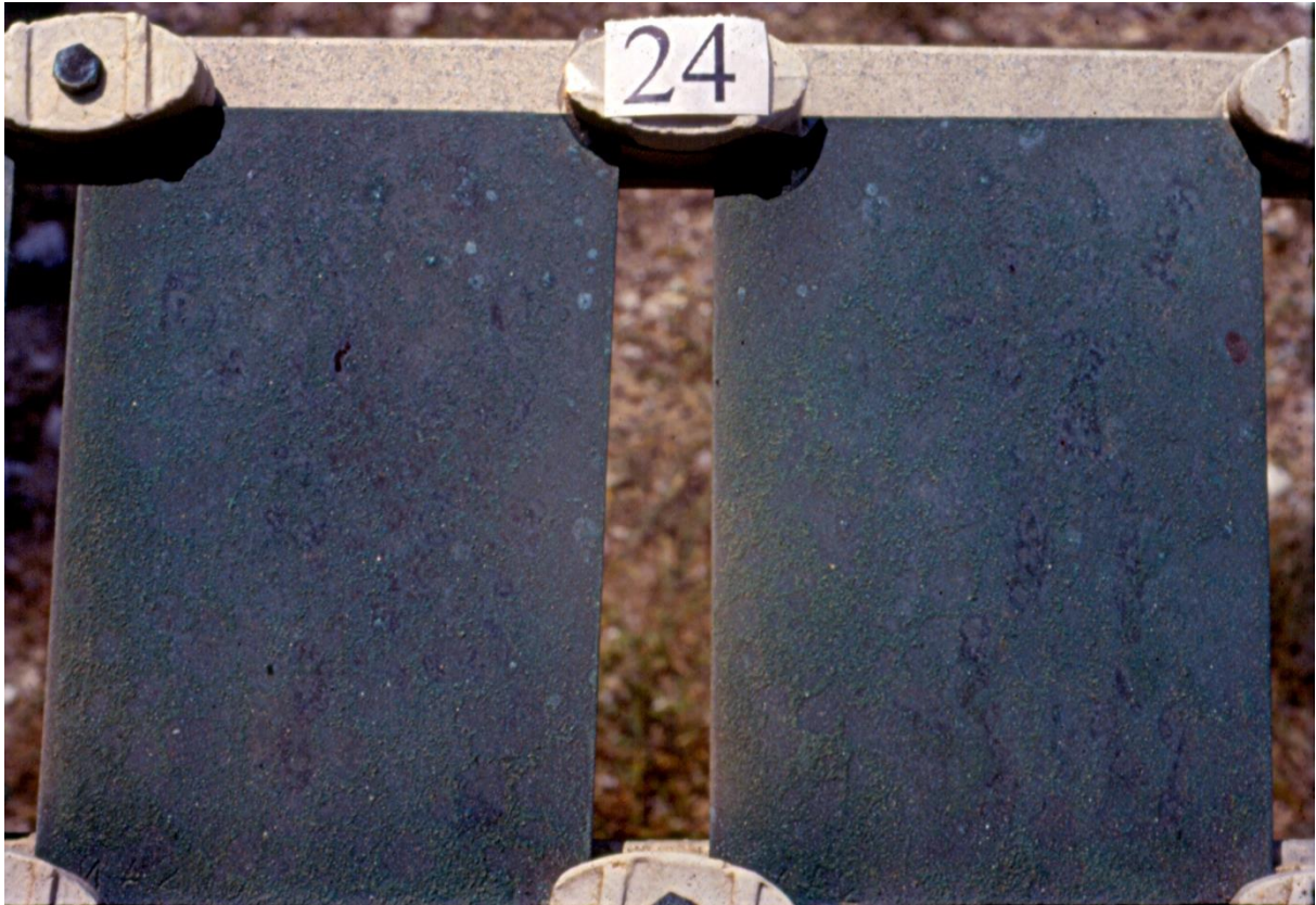
Tarnished Copper of Institute of Metallurgy, Russia exposed at Mandapam for 20 years
