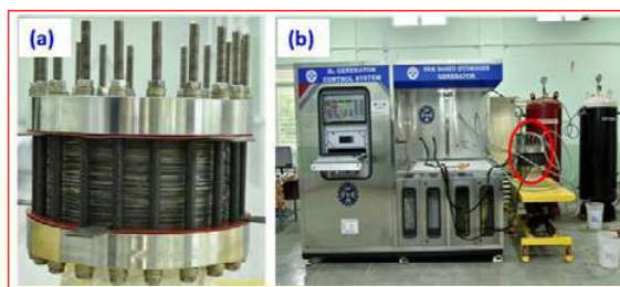
Figure 2. (a) 30 kW stack (b) 30 kW stack integrated with testing unit.
