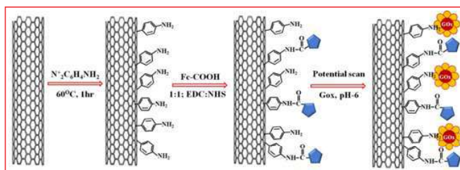
Figure 1. Pictorial representation of the fabrication of bio-anode used for the electrocatalytic glucose oxidation.
