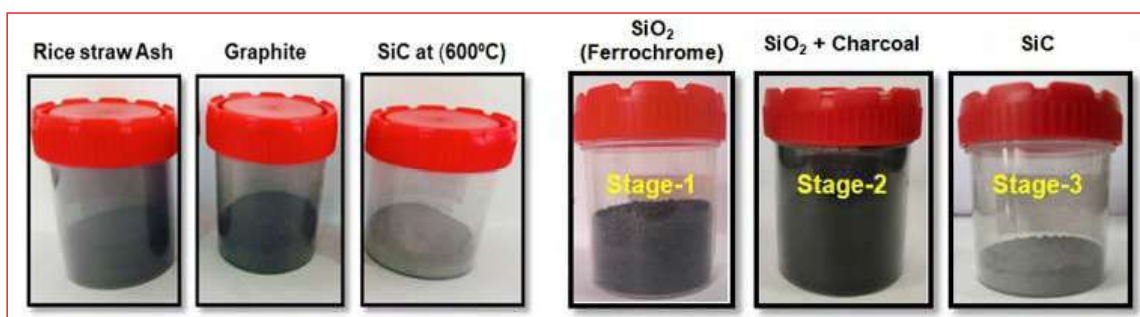
Figure 1. Photographs showing the SiC product obtained from different sources of SiO 2 and Carbon.
