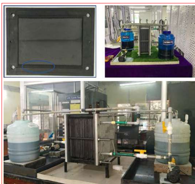
Figure 1. Single moulded gasket for electrolyte flow with sealing solution and AVRFB stacks (12 & 20 cells).
