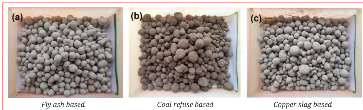
Figure 1. Produced synthetic aggregates based on (a) fly ash, (b) coal refuse, and (c) copper slag.
