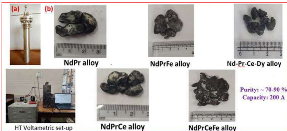
Figure 1. (a) High temperature electrochemical cell (b) RE products from mixture simulating spent magnet composition.
