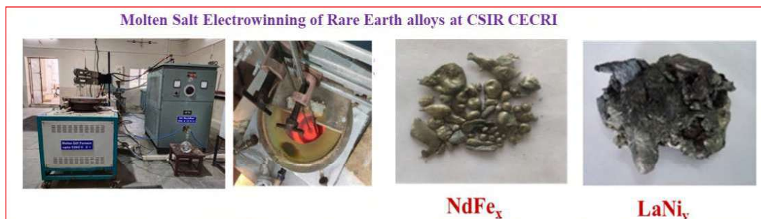
Figure 1. Photographs showing molten salt electrolysis set-up and the products Mg, NdFe x and LaNi y produced.
