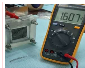
Figure 1. Photograph of in-house assembled aluminium air battery.
