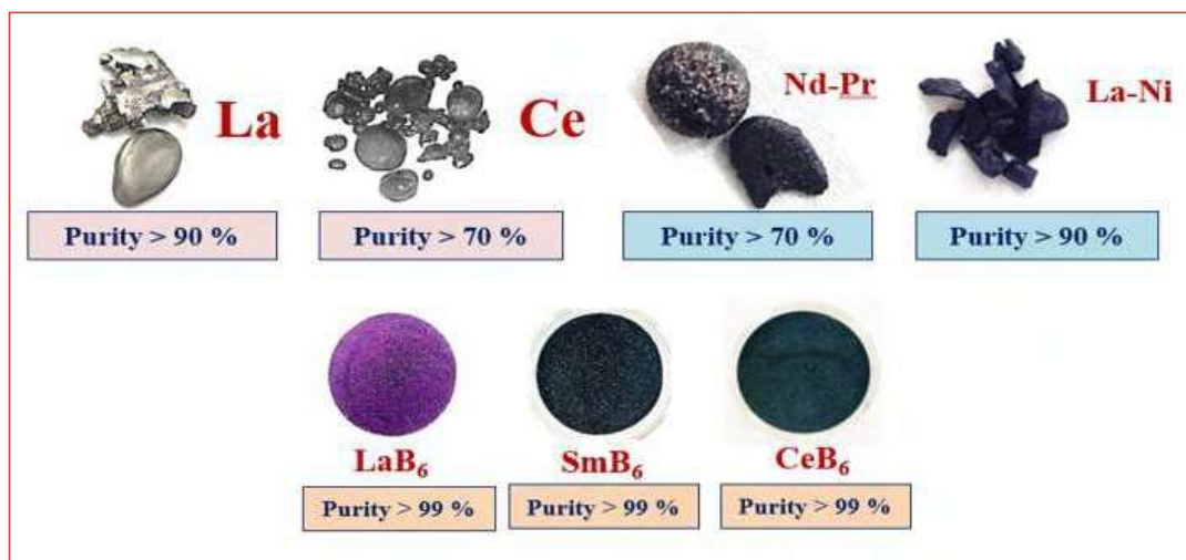
Figure 1. Electrowon RE products through molten salt electrowinning.
