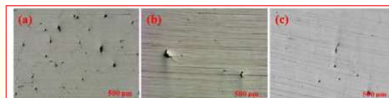
Figure 3. Optical micrographs of Al6063 specimens (a) prior to microalloying and after microalloying using b) 0.5 and c) 1 wt % Ti nano powder.
