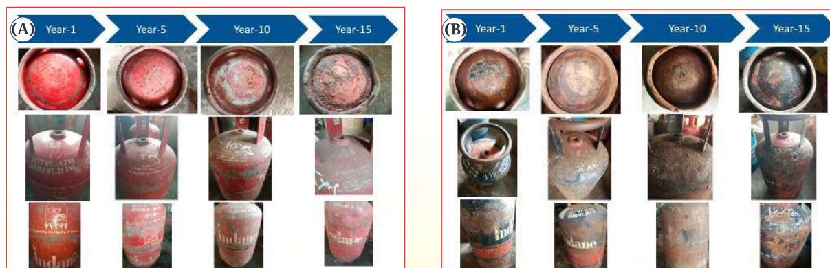
Figure 1. Photograph illustrating progressive corrosion in Domestic (A) and Commercial (B) gas Cylinders.
