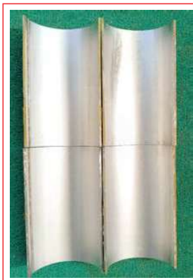
Figure 2. The sectioned chromium plated inner surface of 2 meter tube.
