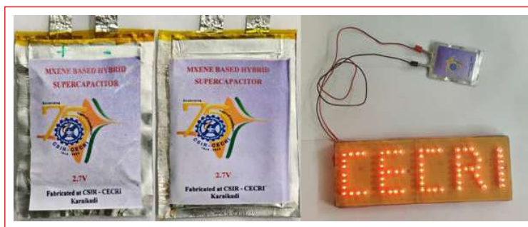
Figure 1. Cyclical galvanostatic charge-discharge. Photographs of fabricated MXene-based hybrid pouch-type supercapacitor and powering an LED arrays by the MXene-based hybrid pouch.
