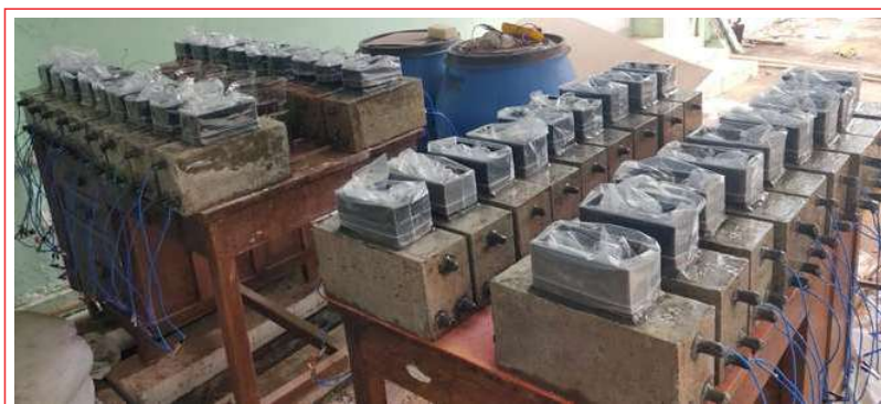
Figure 1. Typical view of macrocell specimens under testing.
