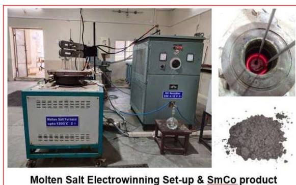
Figure 1. Photographs showing molten salt electrowinning set-up and the obtained SmCo product.
