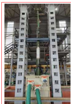
Figure 1. Trivalent hard chromium plating process assembly for 6 meter length gun barrel which was provided by DMRL.
