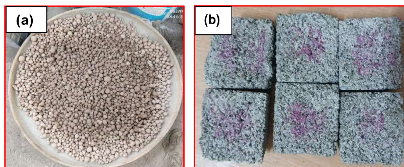
Figure 1. Produced (a) Class C fly ash-based aggregates and (b) Carbonated porous concrete bricks.
