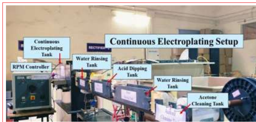
Figure 1. Photograph of existing Nickel plating line.
