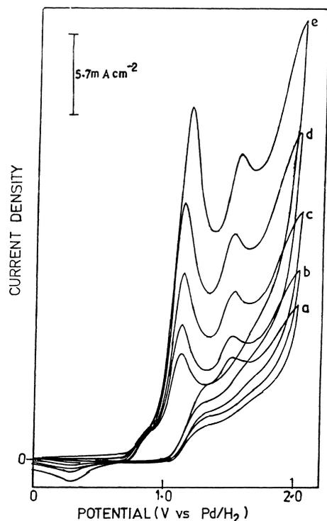
Fig. 2. Cyclic voltammograms for the oxidation of 50 mM of PhSCH<sub>2</sub>COOMe on Pt in Et<sub>3</sub>N·3HF at different  $V$  (mVs<sup>-1</sup>): (a) 20; (b) 40; (c) 80; (d) 160; (e) 320.
