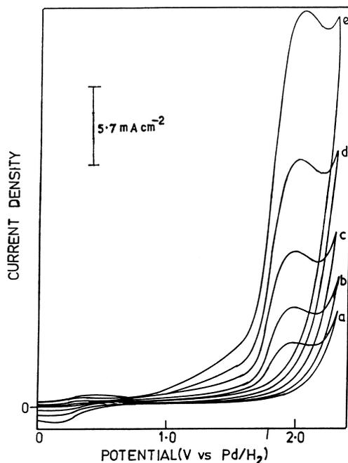
Fig. 1. Cyclic voltammograms for the oxidation of 50 mM of PhCH<sub>2</sub>CN on Pt in Et<sub>3</sub>N·3HF at different  $V$  (mV s<sup>-1</sup>): (a) 20; (b) 40; (c) 80; (d) 160; (e) 320.
