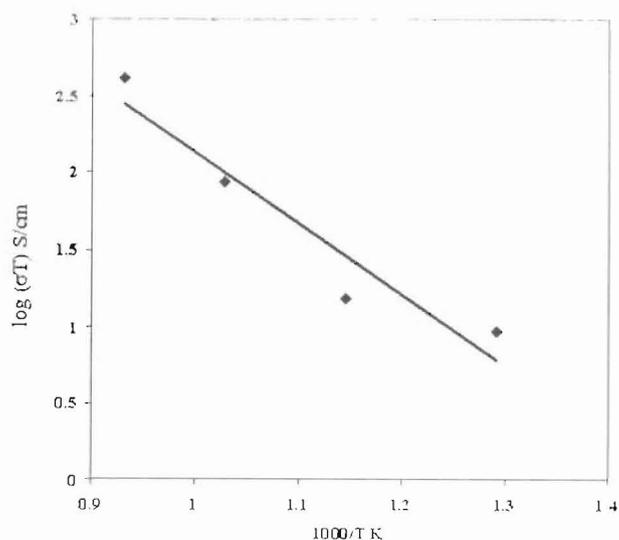
Fig. 6. The effect of temperature on conductivity values of LSC 6535 cathode.
