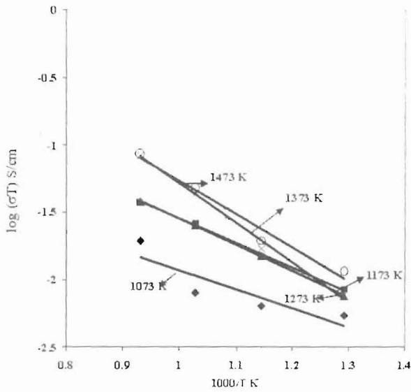
Fig. 7. The effect of temperature on conductivity values of LSC-YZ composite (which were sintered at different temperatures).
