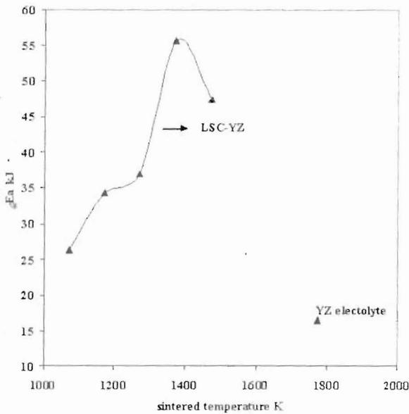
Fig. 8. The influence of sintered temperature on energy of activation of LSC-YZ composite and YZ.
