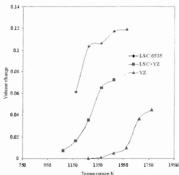
Fig. 4. The effect of temperature on volume change of LSC 6535, YZ and LSC-YZ composite.
