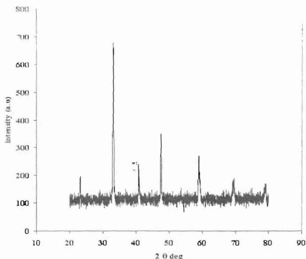
Fig. 1. XRD pattern of LSC 6535 cathode powders.
