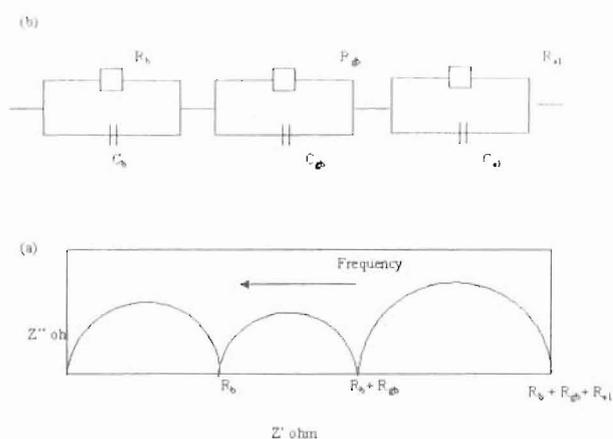
Fig. 5. An idealized equivalent circuit (b) and its corresponding impedance plot (a).  $C_b$ ,  $R_b$  and  $C_{gb}$ ,  $R_{gb}$  and  $C_e$ ,  $R_e$  represents resistance and capacitance for bulk, grain boundary and electrode process, respectively.
