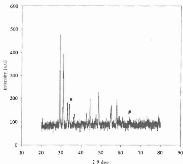
Fig. 2. XRD pattern of LSC 6535-YZ composite powders.
