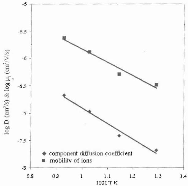
Fig. 10. The effect of temperature on component diffusion coefficient and mobility of ions of LSC-YZ composite.
