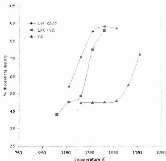
Fig. 3. The effect of temperature on theoretical density of LSC 6535, YZ and LSC-YZ composite.
