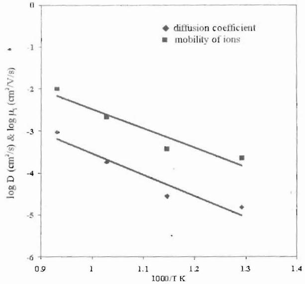
Fig. 9. The effect of temperature on component diffusion coefficient and mobility of ions of LSC 6535 cathode.
