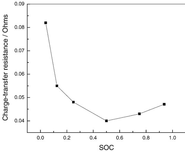
Fig. 5. Charge-transfer resistance values as function of SOC for Pb|PbSO<sub>4</sub> electrode of 6-V/4-Ah lead–acid battery.
