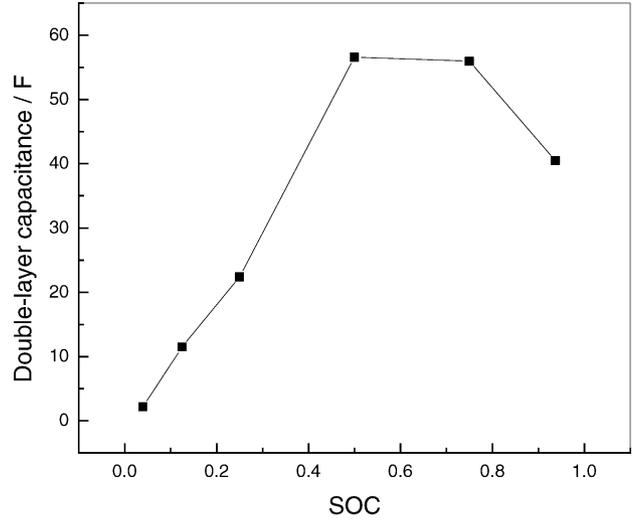
Fig. 8. Double-layer capacitance values as function of SOC for Pb|PbSO<sub>4</sub> electrode of 6-V/4-Ah lead–acid battery.
