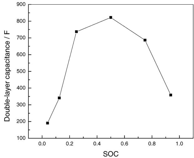
Fig. 9. Double-layer capacitance values as function of SOC for PbO<sub>2</sub>|PbSO<sub>4</sub> electrode of 6-V/4-Ah lead–acid battery.
