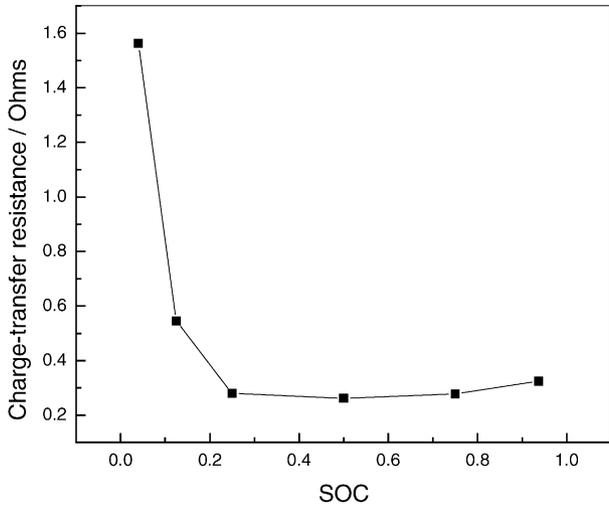
Fig. 6. Charge-transfer resistance values as a function of SOC for PbO<sub>2</sub>|PbSO<sub>4</sub> electrode of 6-V/4-Ah lead–acid battery.
