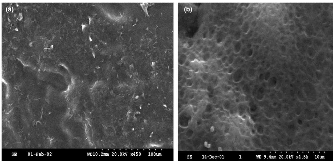
Fig. 2. SEM micrograph of: (a) PAN-PTSA/CMC reinforced conducting E-glass fabric; (b) PAN-CSA/CMC reinforced conducting E-glass fabric.
