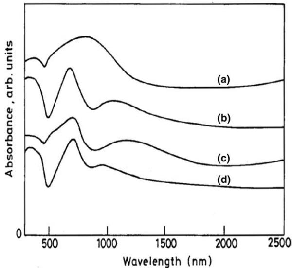
Fig. 1. UV-Vis-NIR absorption spectra of: (a) PAN-PTSA/CMC reinforced conducting E-glass fabric; (b) PAN-PTSA grafted E-glass fabric; (c) PAN-CSA/CMC reinforced conducting E-glass fabric; (d) PAN-CSA grafted E-glass fabric.
