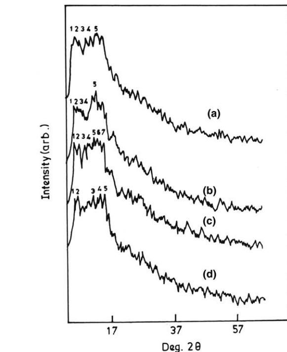
Fig. 3. X-ray diffraction powder pattern (Cu  $K\alpha$ ,  $\lambda = 1.5418\ \text{\AA}$ ) of: (a) PAN–PTSA grafted E-glass fabric; (b) PAN–PTSA/CMC reinforced conducting E-glass fabric; (c) PAN–CSA grafted E-glass fabric; (d) PAN–CSA/CMC reinforced conducting E-glass fabric.
